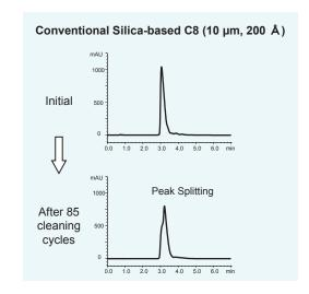
Repeat sample injections may induce adsorption of proteins, which could result in the loss of retention and/or loss of resolution of the target molecule.
