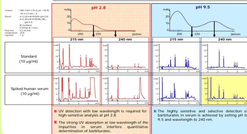
UV detection with low wavelength is required for high-sensitive analysis at pH 2.8. The strong UV absorption at low wavelength of the impurities in serum interfere quantitative determination of barbiturates.
