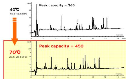
23% more peaks can be resolved by increasing the column temperature to 70°C in peptide mapping.
