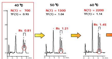
The column temperature is increased at pH 7.9, and the higher temperature provides sharper peaks.
