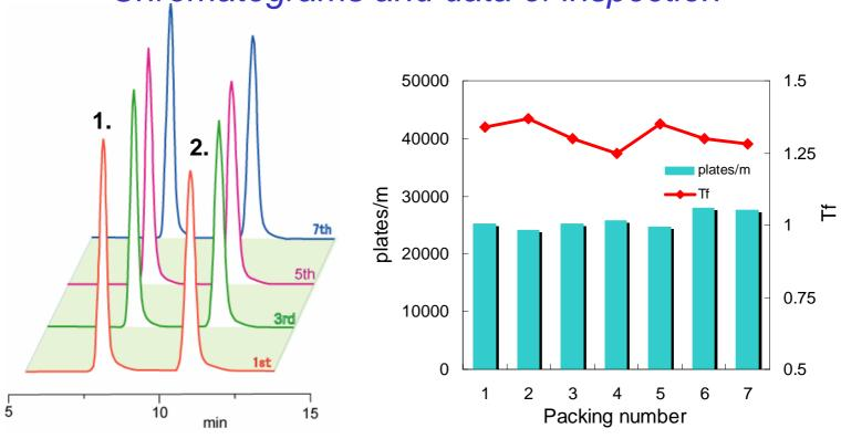
By using a 50 mml.D. DAU column, repacking procedure was attempted. After 7 times repacking, plates/m and Tf are still good as the initial state.
