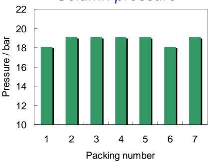
Eluent: methanol/water (85/15), Flow rate: 150 mL/min
