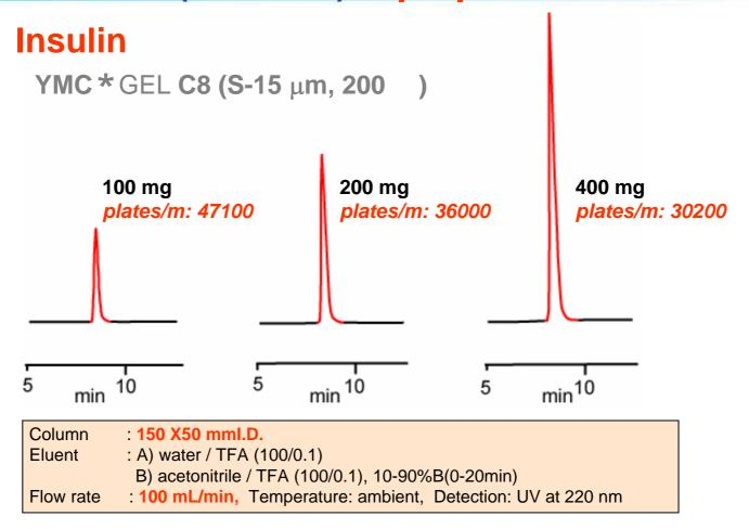
Up to 400 mg loaded amount, peak shapes are sharp as the analytical separation.
