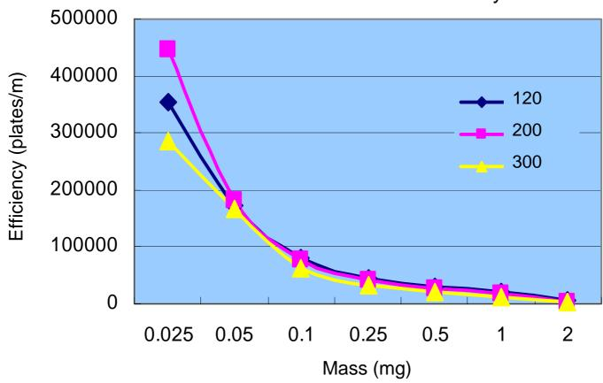
pore size is the best choice for samples up to the **200** 0.1 mg loading level.
