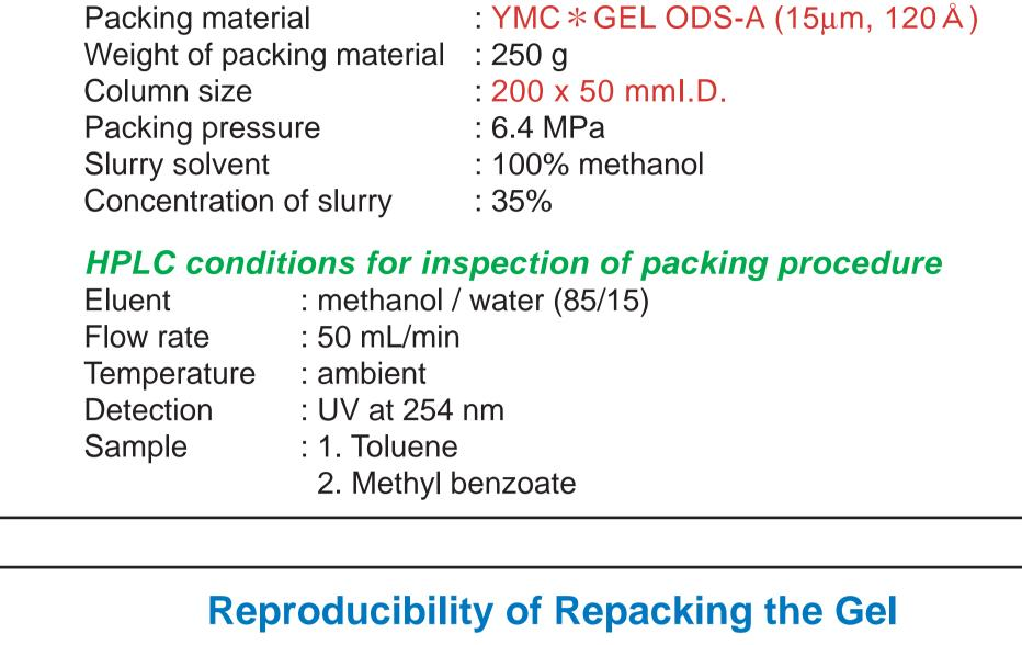
Optimum Packing Conditions for 50 mml.D. DAU Column
