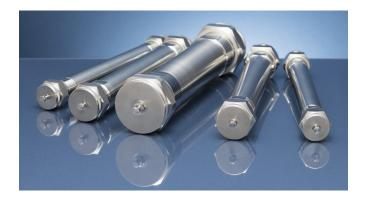
YMC-Actus preparative columns were developed by applying this same technology. The column bed is compressed when attaching the inlet end assembly of the YMC-Actus hardware. This provides increased bed density (10% higher than that of conventional columns) and bed uniformity. Packed with YMC resins, Actus columns have been shown to maintain high stability under high flow rates and steep gradient conditions.
