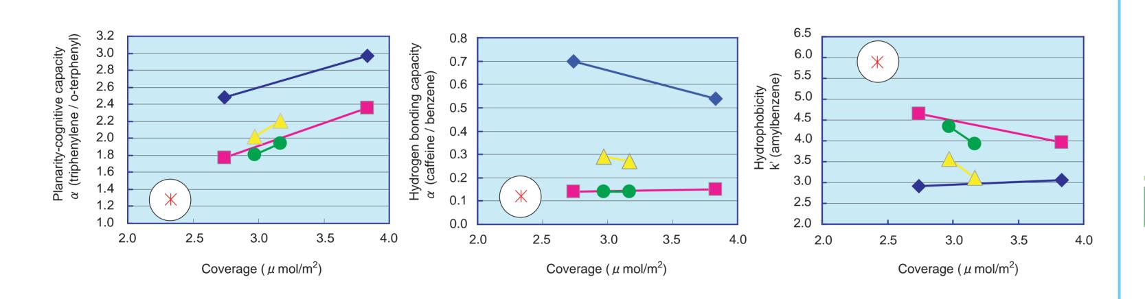
In the polymeric materials, the planarity-cognitive capacity is getting higher with increasing carbon coverage. Especially, non-endcapped polymeric material show higher value than endcapped material.
