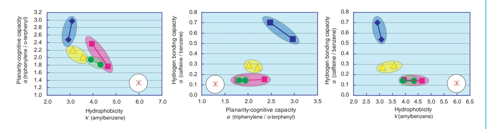
As compared with the standard-type ODS (monomeric / endcapped, marked with \* in the figures), the materials used in this study show great differences in the fundamental separation properties. When not endcapped, the difference between the polymeric-type and monomeric-type are particularly significant. These differences suggest a possibility that some compounds hardly separable with the standard-type ODS may be separated favorably with these materials peculiar characteristics.
