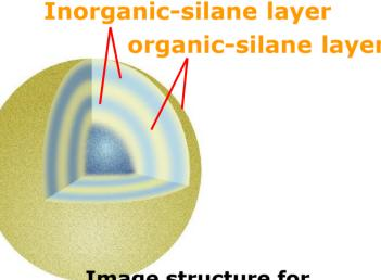
Image structure for hybrid-silica particle
