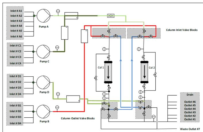
Fig. 4: Basic schematic of Contichrom TWIN HPLC for MCSGP
