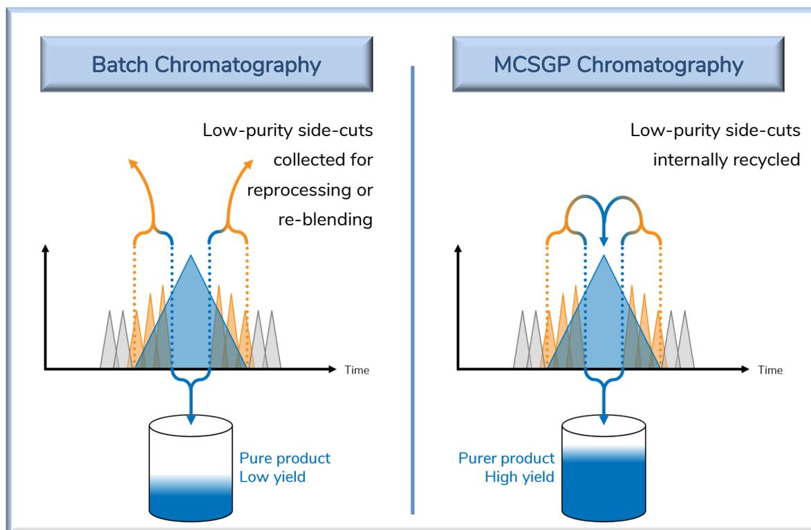
Fig. 3: Conventional single-column batch chromatography is restricted to a narrow center cut of target molecule to achieve adequate yield. MCSGP, on the other hand, continuously recycles the side fractions to achieve both high purity and high yield of the target.
