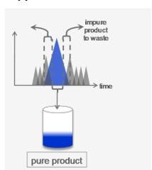
A typical batch process collects the pure portion of the desired peak. The portions with early and late impurities are discarded or retained for later reprocessing.
