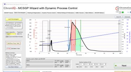
The Wizard makes an initial prediction for the chromatographic method. Adjustments can be made to sample loading, flow rates, column washes and equilibration steps parameters.
