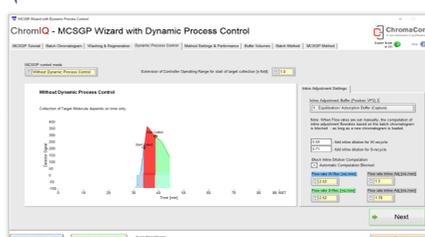
The number of cycles, maximum system pressure and how the collected product is pooled are set within the Wizard. The Wizard also makes predictions for the expected method performance.
