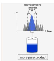
An MCSGP process collects the pure portion of the desired peak. The portions with early and late impurities are sent to a second column while adding more feed material and the purification continues.
