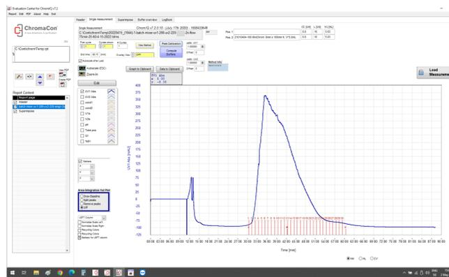
A single column, linear gradient batch run is made on a CUBE. There must be a segment of the desired peak with suitable purity. Fractions are collected that capture all of the desired material.
