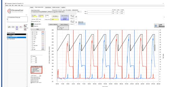
The MCSGP data can also be displayed as an overlay of the different cycles. The shaded areas represent the portions that are the early eluting recycled portion, the collected portion and the late eluting recycled portion.
