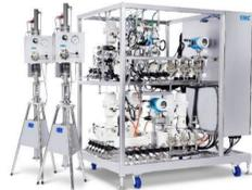
Custom built production equipment with flowrates up to 40 L/min. Capable of running MCSGP, single column batch, and separately - CaptureSMB.
