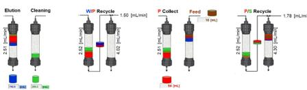
The left column running a sample while the right column is being cleaned. Recycling the impure early eluting portion. Collecting the pure portion and adding more feed to the second column. Recycling the impure late eluting portion. The next step would be the right column running a sample while the left column is being cleaned.
