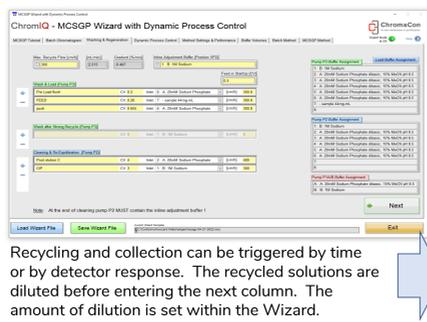
Recycling and collection can be triggered by time or by detector response. The recycled solutions are diluted before entering the next column. The amount of dilution is set within the Wizard.
