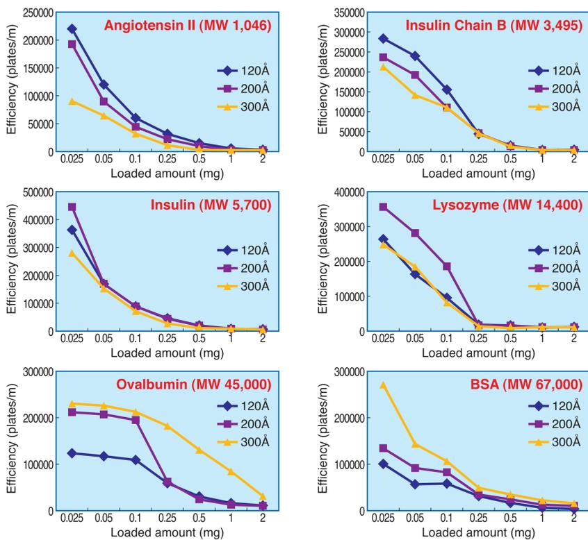
In the case of low molecular weight peptides up to MW 3,500, 120 Å pore size (◆) is most efficient at all the loading levels. Large peptides and small proteins such as Insulin and Lysozyme are adapted to 200 Å pore size (■) at relatively low loading levels. In separation of proteins larger than MW 40,000, 300 Å pore size (▲) gives the highest efficiency. 120 Å and 200 Å pore sizes would be too small to give a good peak shape and resolution.
