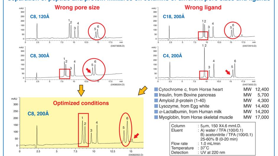
These chromatograms show an optimization of separation of large peptide and small protein mixtures (MW 4,300 ~ 17,000) on the columns of different pore sizes and ligands. The combination of appropriate pore size and hydrophobicity of bonding chemistry, 200 Å C8, yields the best resolutions and peak shapes.
