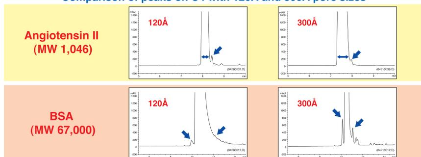
It is important to choose an appropriate pore size for achieving a good peak shape. An overly small or overly large pore size results in peak broadening and poor resolution.
