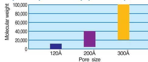
The 120 Å pore size is ideal for peptides with a MW ranging from 200 to 10,000. The 200 Å pore size is ideal for large peptides and small proteins with a MW ranging from 5,000 to 40,000. The 300 Å pore size is suitable to proteins with a MW of ≥ 20,000.
