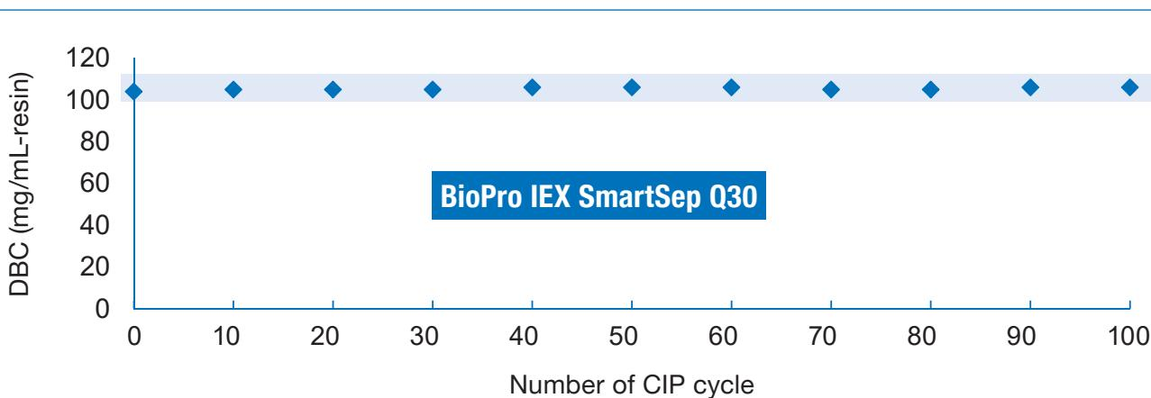
**BioPro IEX SmartSep S30 and Q30 maintain their binding capacity even after 100 CIP cycles.**
