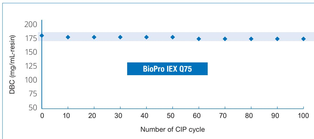
**BioPro IEX S75 and Q75 maintain their binding capacity even after 100 CIP cycles.**
