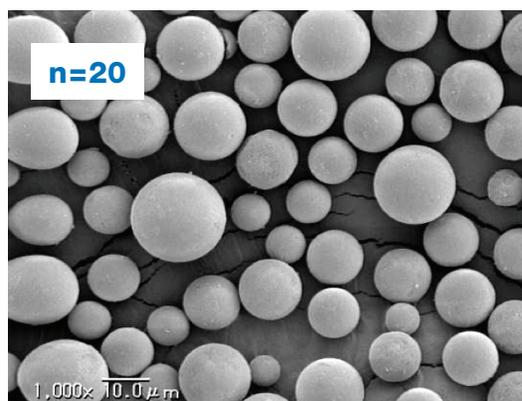
SEM pictures of the material before the first packing and after the 20<sup>th</sup> packing prove the high mechanical stability of the YMC-Triart Prep materials.
