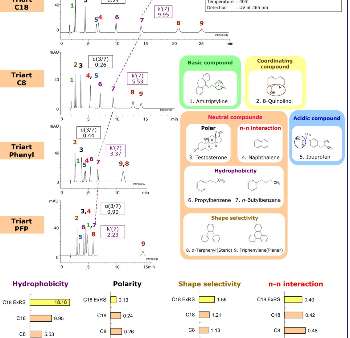
■ The retention behavior of Triart RP columns is compared in the separation of nine compounds illustrated in above. The compounds are selected as indicators of several types of chromatographic properties, such as hydrophobicity, polar and π-π interactions, shape selectivity, retention and peak shapes for ionic compounds. These chromatograms show each bonded phase has different capacity and selectivity.
