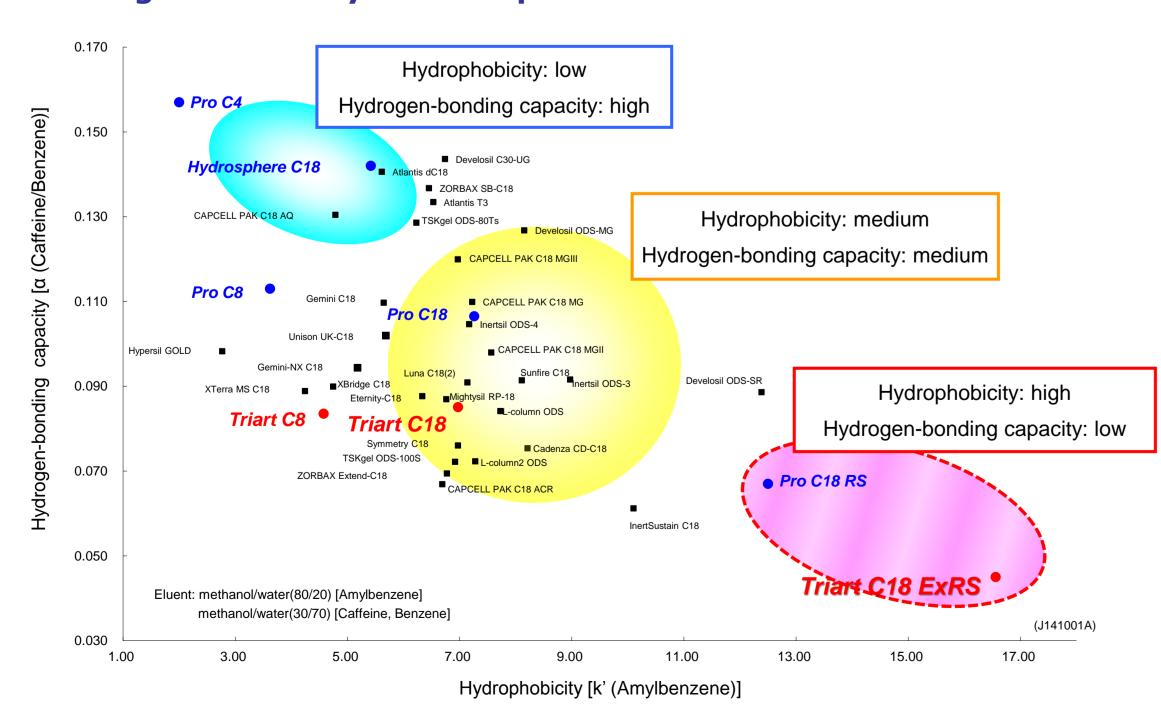
Triart C18 ExRS has significantly higher hydrophobicity and lower hydrogen-bonding capacity than a lot of commercial C18 phases. This unique selectivity is provided by high-coverage C18 phases bonded to hybrid particles with large surface area and it complements a standard Triart C18 and other RP columns especially in separation of hydrophobic compounds with similar structure.
