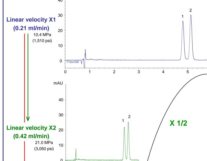
As shown in above chromatograms, HPLC method of Vitamin D<sub>2</sub> and D<sub>3</sub> separation using 5 µm Triart C18 ExRS column is transferred to UHPLC method using 1.9 µm column with similar L/dp (ratio of column length to particle diameter).
