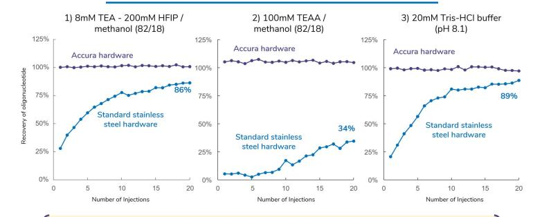
The YMC-Accura hardware with its inert column surface prevents adsorption of oligonucleotides regardless of buffer type. Conditioning injections of sample are not required, ensuring high recovery and reproducibility from the very first use. In addition, YMC-Accura columns provide significantly higher recoveries and sensitivities that cannot be achieved with standard stainless steel columns – even after conditioning the standard columns with 20 sample injections.
