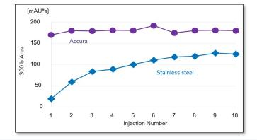
YMC-Accura Triart Bio C4 shows stable peak area from the first injection, while the standard stainless steel column provides only 1/10 of the peak area at the first injection. Even after the tenth injection, the peak area of the stainless steel column is considerably less than that of the Accura column.
