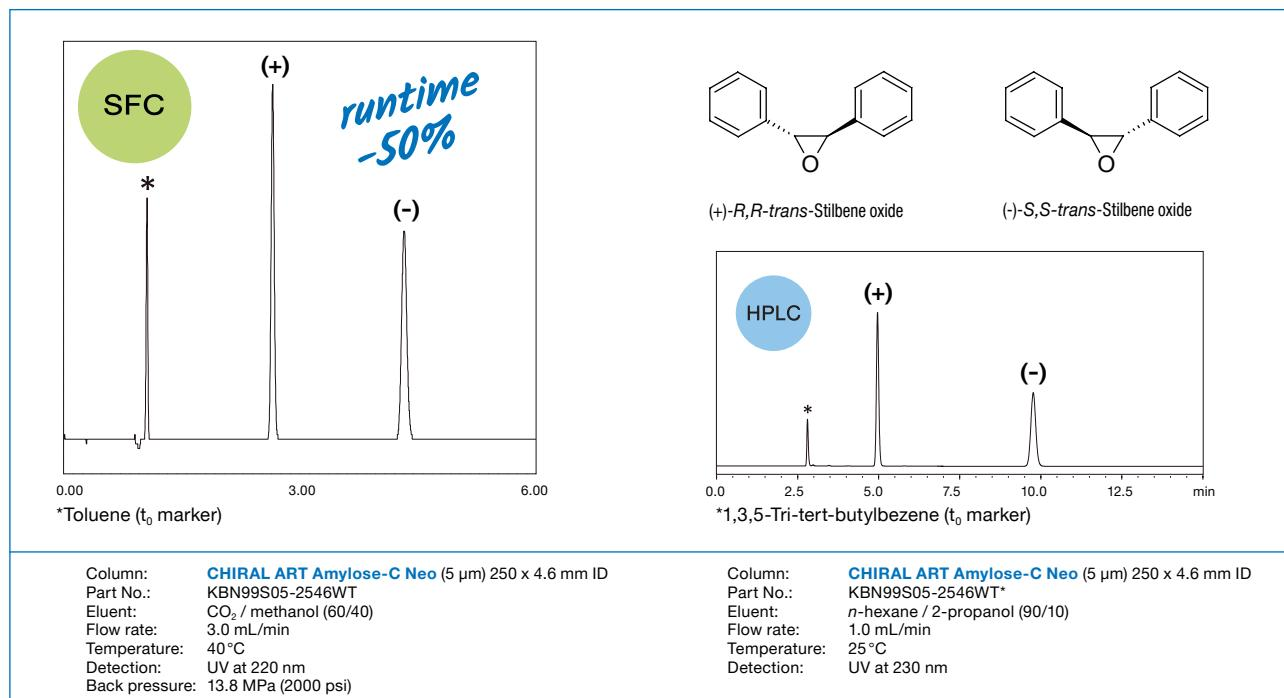
Faster chiral separation of trans-stilbene oxide is achieved using supercritical fluid chromatography compared to HPLC as the separation mode. Lower viscosity and larger diffusion coefficients for supercritical fluid provide rapid separations of both chiral and achiral compounds.
