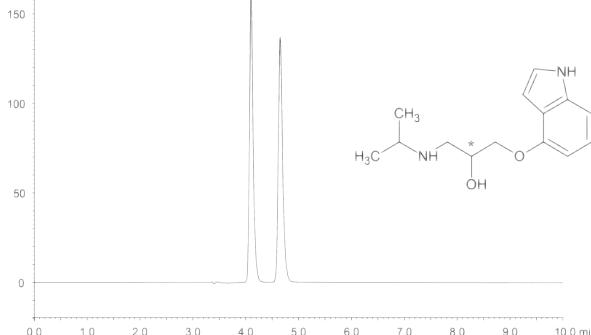
Column: CHIRAL ART Cellulose-SB (5  $\mu$ m) 250 x 4.6 mm ID
