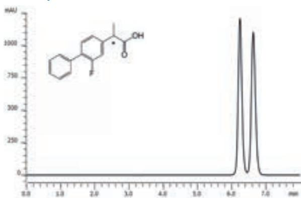
Column: CHIRAL ART Cellulose-C (5 µm) 250 x 4.6 mm ID
