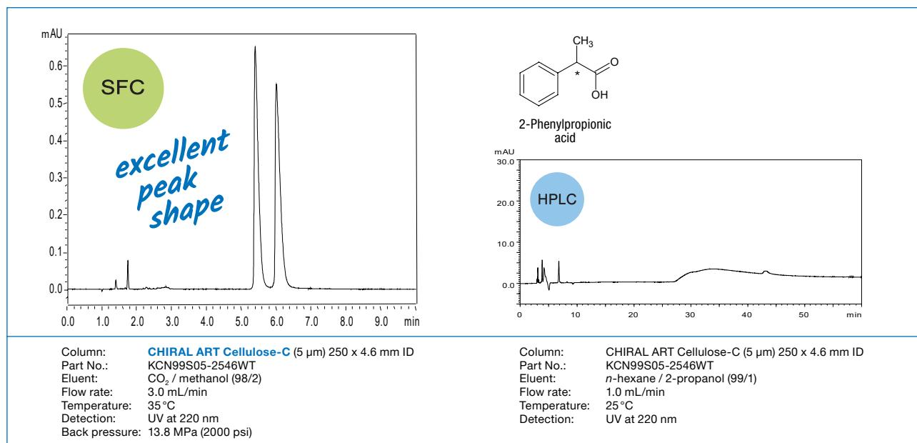
Excellent peak shape of 2-phenylpropionic acid is obtained using SFC chiral separation. Under HPLC conditions, the peak shape is very broad with mobile phase containing no additives such as an acid. With SFC, on the other hand, peak shapes are very good just with a mixture of  $\text{CO}_2$  and methanol. It is thought that supercritical carbon dioxide acts as a weak acid.
