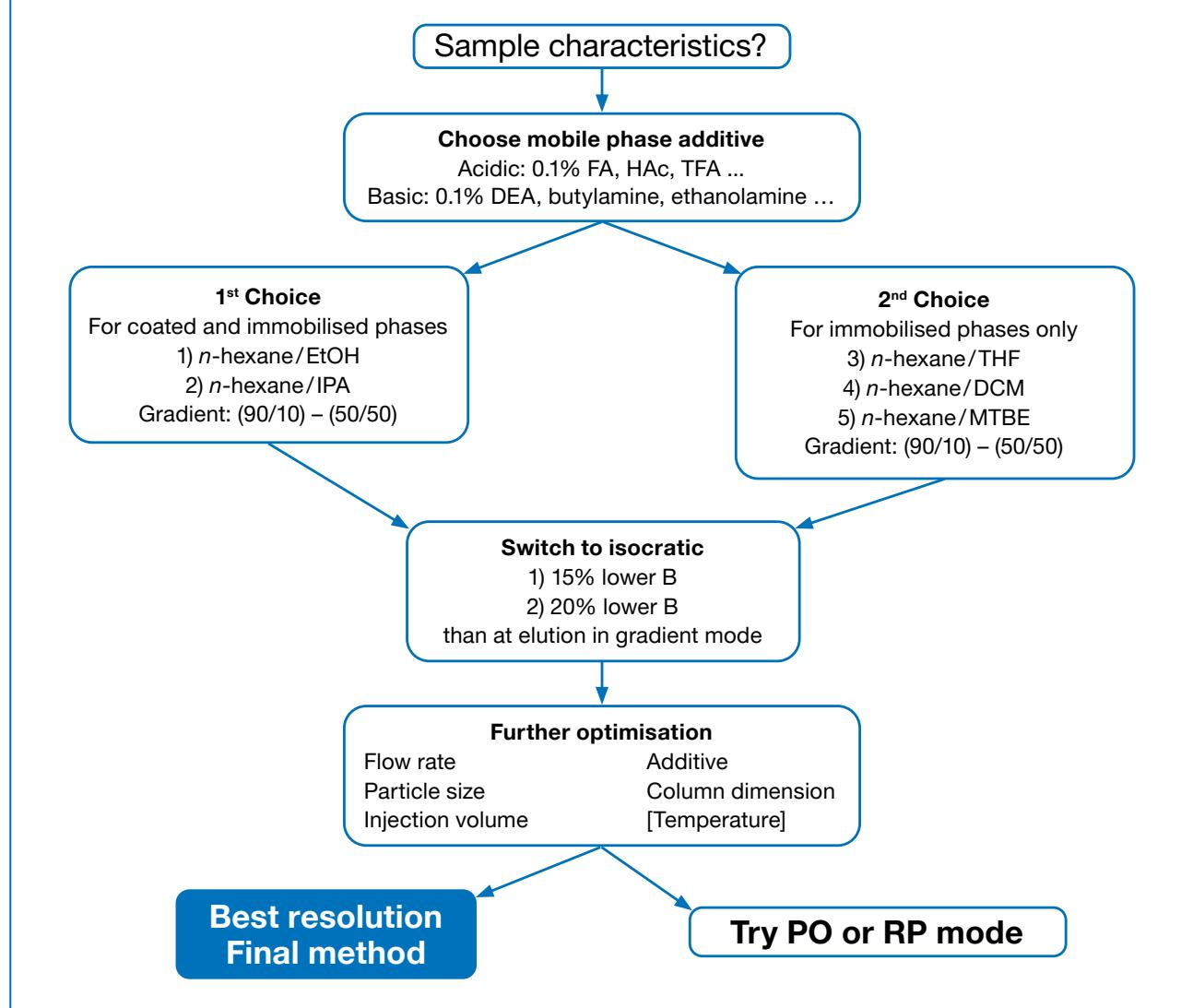
For Polar Organic (PO) mode, methanol, ethanol or mixtures of both can be used as well as acetonitrile or mixtures of methanol and acetonitrile. RP mode can only be applied to immobilised polysaccharide phases.
