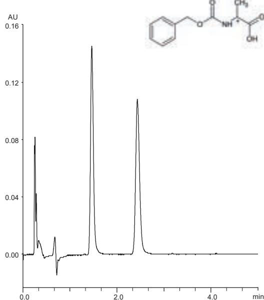
Column: CHIRAL ART Amylose-C Neo (3 µm) 50 x 3.0 mm ID
