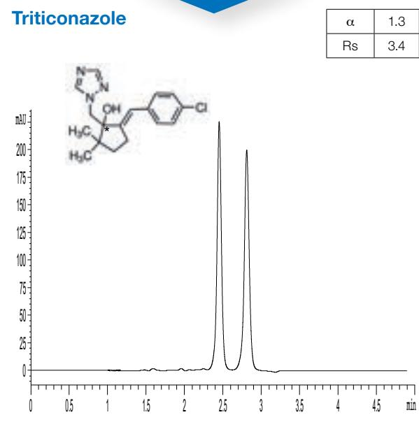
Column: CHIRAL ART Cellulose-SB (3  $\mu$ m) 150 x 3.0 mm ID
