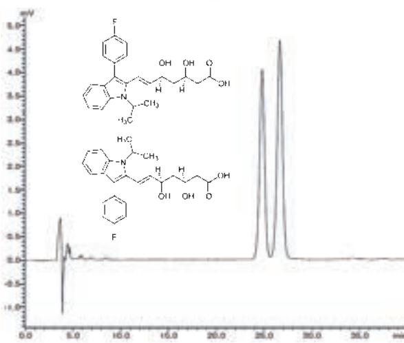
Column: CHIRAL ART Cellulose-SB (5 µm) 250 x 4.6 mm ID
