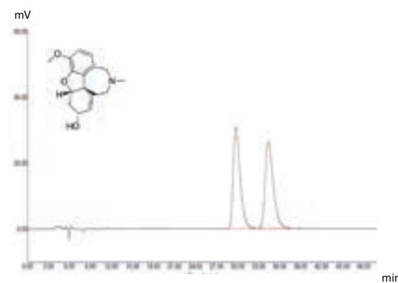
Column: CHIRAL ART Amylose-C\* (5 µm) 250 x 4.6 mm ID
