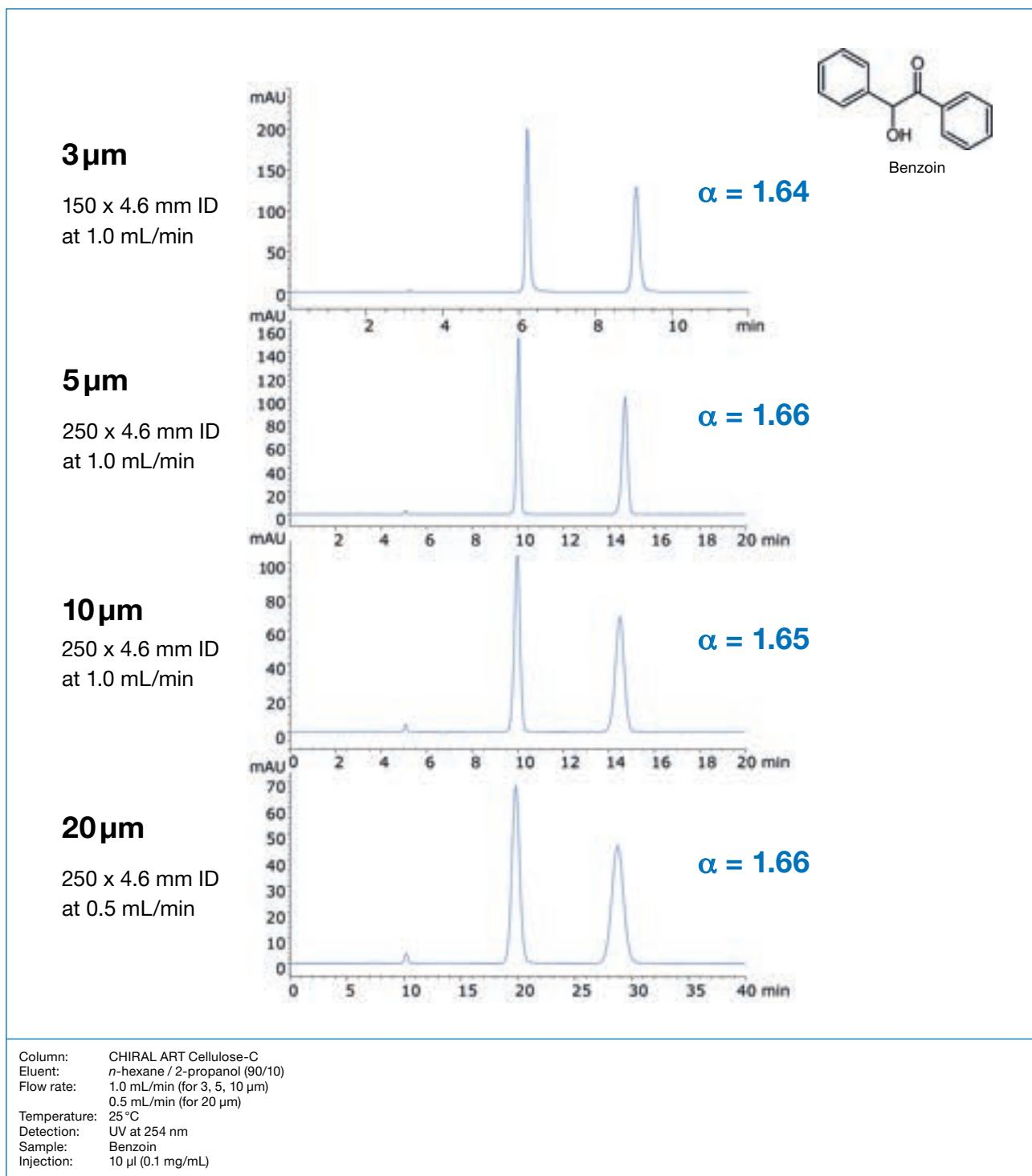
CHIRAL ART shows identical selectivity and excellent peak shapes for materials with particle sizes from 3  $\mu\text{m}$  to 20  $\mu\text{m}$ . It allows predictable scale up from analytical LC to semi-preparative or preparative LC, and vice versa. Screening and method development can be done on small particle sizes and the results can easily be transferred to larger particle sizes.
