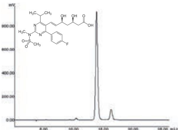
Column: CHIRAL ART Cellulose-SB (5  $\mu$ m) 250 x 4.6 mm ID
