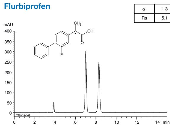
Column: CHIRAL ART Amylose-SA (5 µm) 250 x 4.6 mm ID
