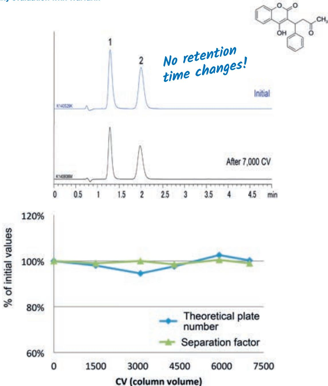
Column: CHIRAL ART Amylose-C\* (5 µm) 50 x 3.0 mm ID
