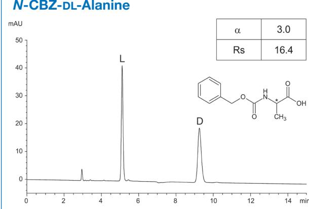
Column: CHIRAL ART Cellulose-C (5  $\mu$ m) 250 x 4.6 mm ID
