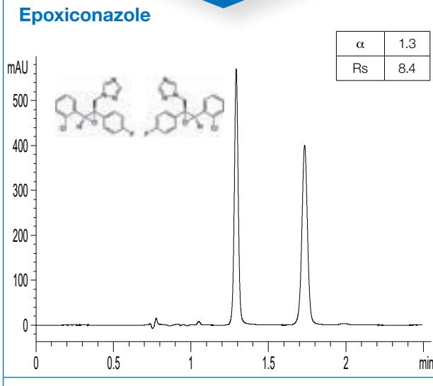
Column: CHIRAL ART Cellulose-SB (3  $\mu$ m) 150 x 3.0 mm ID
