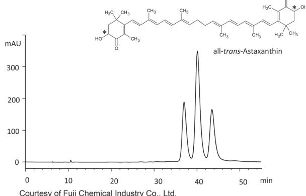
Column: CHIRAL ART Cellulose-SB (5 µm) 250 x 4.6 mm ID
