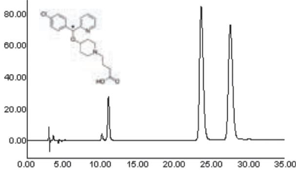
Column: CHIRAL ART Amylose-SA (5 µm) 250 x 4.6 mm ID
