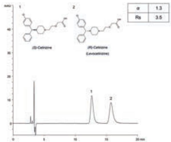
Column: CHIRAL ART Cellulose-C (5 µm) 250 x 4.6 mm ID
