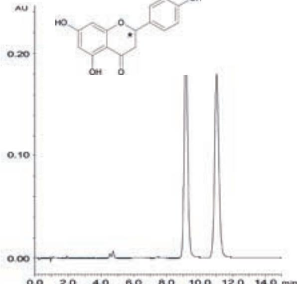
Column: CHIRAL ART Cellulose-SB (5 µm) 250 x 4.6 mm ID
