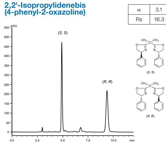
Column: CHIRAL ART Amylose-C Neo (5 µm) 250 x 4.6 mm ID
