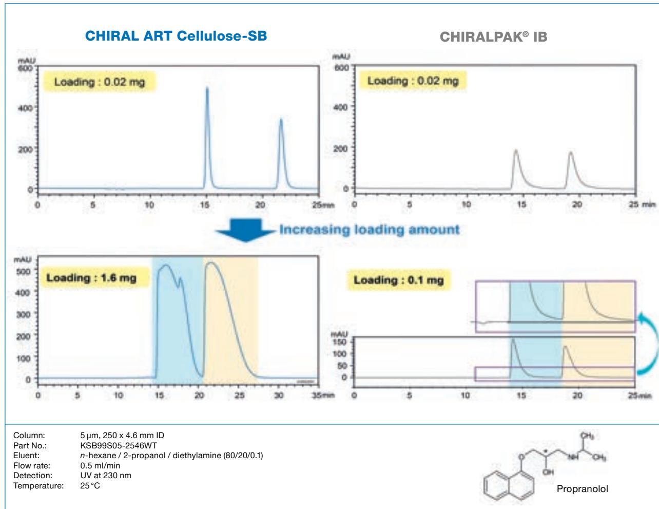
For the competitor's product, loading amount of more than 0.1 mg was not possible because the enantiomeric excess of the 2<sup>nd</sup> peak was already less than 98%ee with a loading amount of 0.1 mg.
