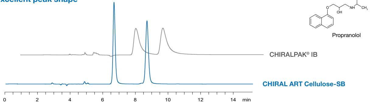
**CHIRAL ART polysaccharide derivatives provide excellent peak shapes for ionic and metal coordinating compounds.**
