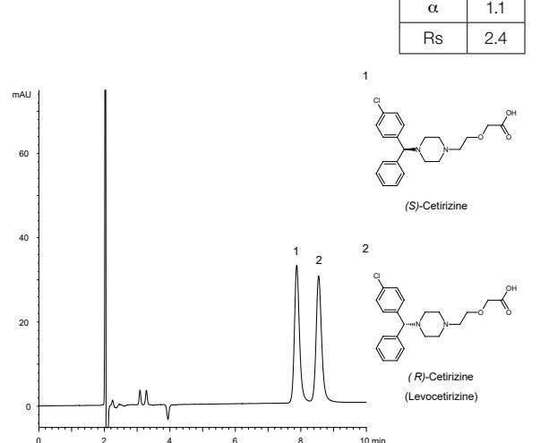
Column: CHIRAL ART Cellulose-SB (3 µm) 150 x 4.6 mm ID
