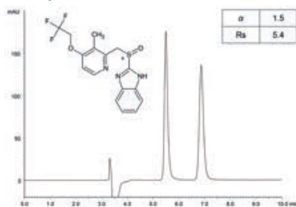
Column: CHIRAL ART Amylose-SA (5 µm) 250 x 4.6 mm ID
