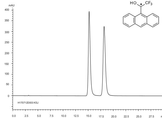
Column: CHIRAL ART Cellulose-SJ (5 µm) 250 x 4.6 mm ID
