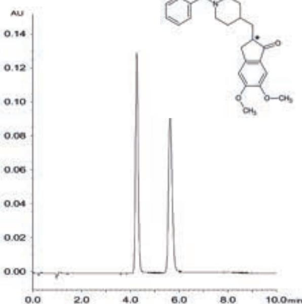
Column: CHIRAL ART Cellulose-C (5 µm) 250 x 4.6 mm ID
