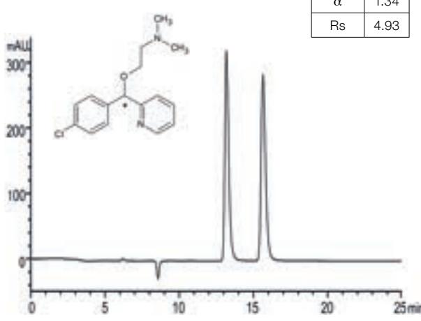
Column: CHIRAL ART Amylose-SA (5 µm) 250 x 4.6 mm ID
