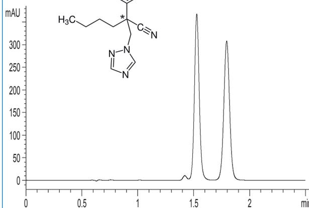
Column: CHIRAL ART Cellulose-SB (3  $\mu$ m) 50 x 4.6 mm ID
