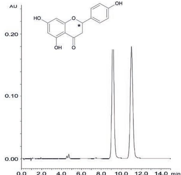
Column: CHIRAL ART Cellulose-SB (5  $\mu$ m) 250 x 4.6 mm ID
