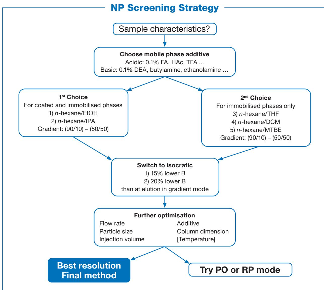
For Polar Organic (PO) mode, methanol, ethanol or mixtures of both can be used as well as acetonitrile or mixtures of methanol and acetonitrile. RP mode can only be applied to immobilised polysaccharide phases.
