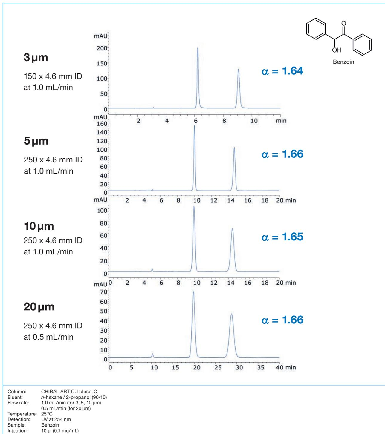
CHIRAL ART shows identical selectivity and excellent peak shapes for materials with particle sizes from 3  $\mu\text{m}$  to 20  $\mu\text{m}$ . It allows predictable scale up from analytical LC to semi-preparative or preparative LC, and vice versa. Screening and method development can be done on small particle sizes and the results can easily be transferred to larger particle sizes.
