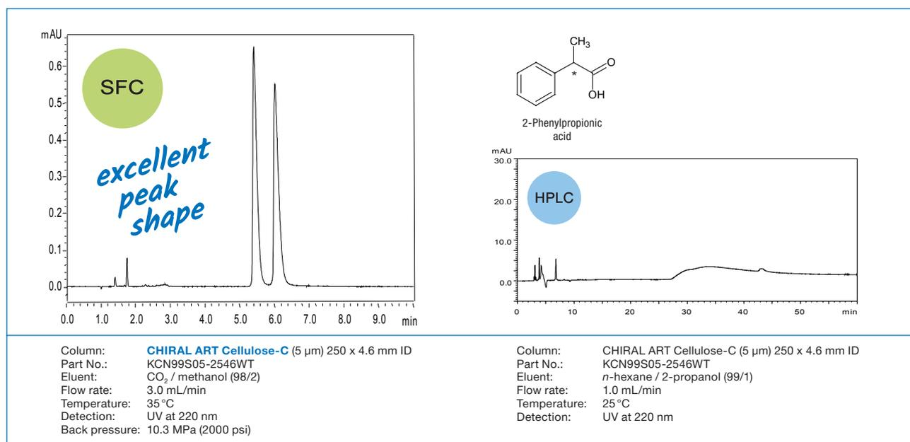
Excellent peak shape of 2-phenylpropionic acid is obtained using SFC chiral separation. Under HPLC conditions, the peak shape is very broad with mobile phase containing no additives such as an acid. With SFC, on the other hand, peak shapes are very good just with a mixture of CO<sub>2</sub> and methanol. It is thought that supercritical carbon dioxide acts as a weak acid.
