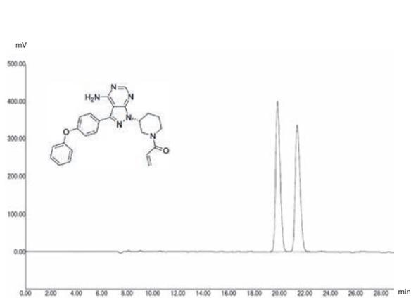
Column: CHIRAL ART Cellulose-C (5  $\mu$ m) 250 x 4.6 mm ID
