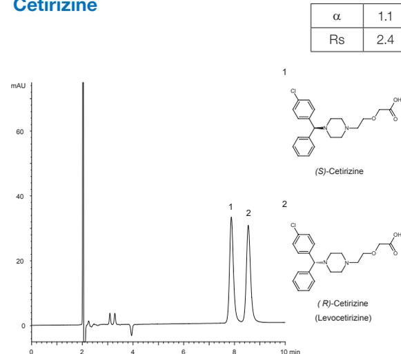
Column: CHIRAL ART Cellulose-SB (3  $\mu$ m) 150 x 4.6 mm ID
