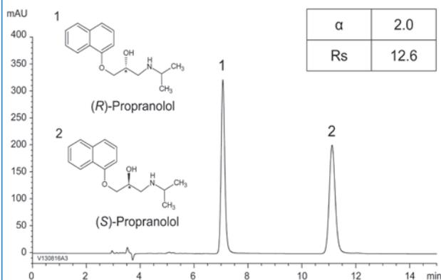
Column: CHIRAL ART Cellulose-C (5  $\mu$ m) 250 x 4.6 mm ID
