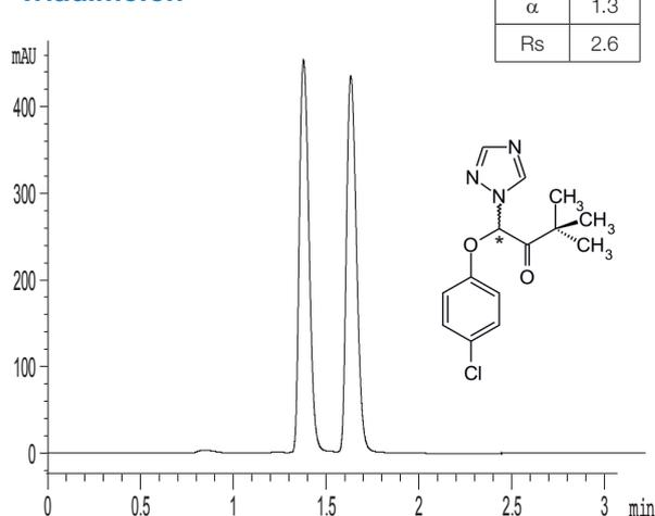
Column: CHIRAL ART Cellulose-C (3  $\mu$ m) 150 x 3.0 mm ID
