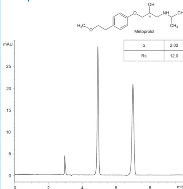
Column: CHIRAL ART Cellulose-C (5  $\mu$ m) 250 x 4.6 mm ID
