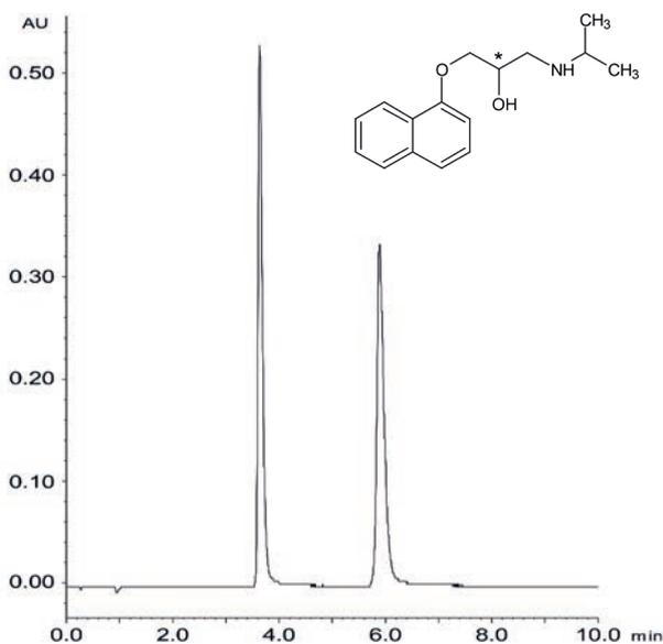
Column: CHIRAL ART Cellulose-C (5  $\mu$ m) 250 x 4.6 mm ID
