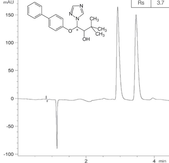
Column: CHIRAL ART Cellulose-C (3  $\mu$ m) 150 x 3.0 mm ID
