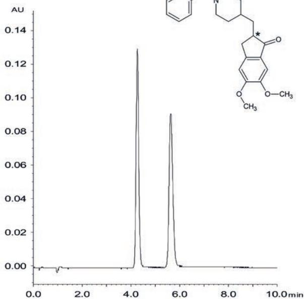
Column: CHIRAL ART Cellulose-C (5  $\mu$ m) 250 x 4.6 mm ID
