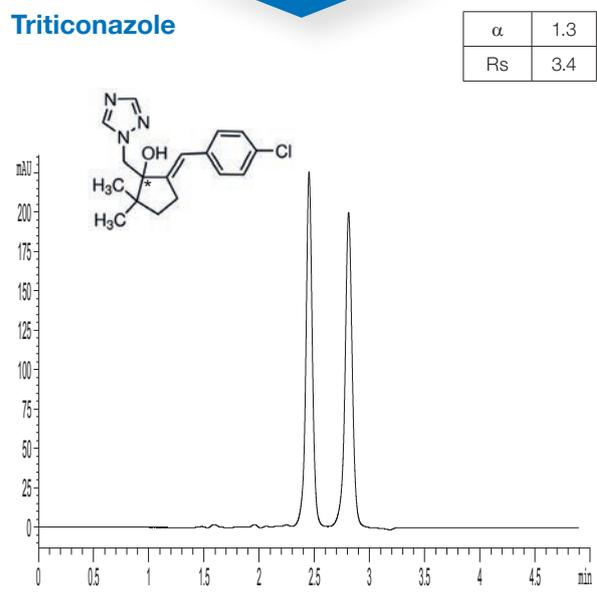
Column: CHIRAL ART Cellulose-SB (3  $\mu$ m) 150 x 3.0 mm ID
