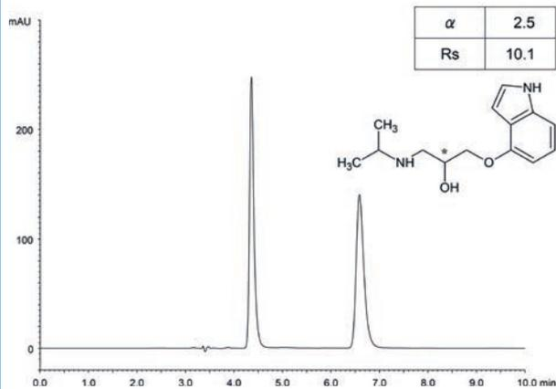
Column: CHIRAL ART Cellulose-SB (5  $\mu$ m) 250 x 4.6 mm ID
