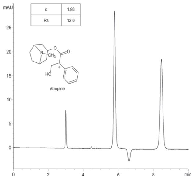
Column: CHIRAL ART Cellulose-C (5  $\mu$ m) 250 x 4.6 mm ID
