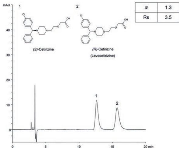
Column: CHIRAL ART Cellulose-C (5  $\mu$ m) 250 x 4.6 mm ID
