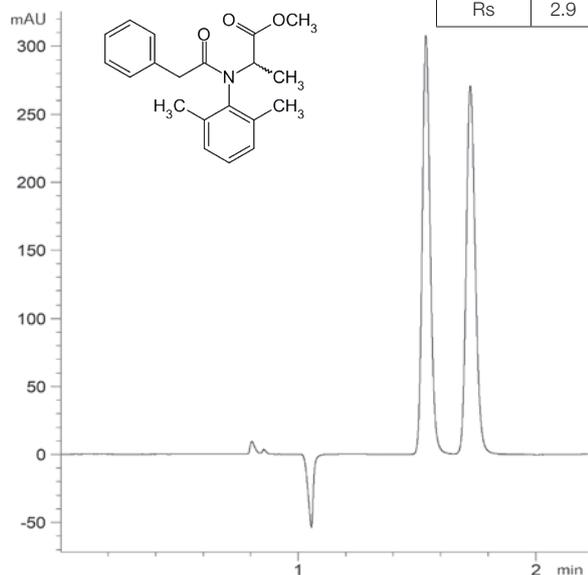
Column: CHIRAL ART Cellulose-C (3  $\mu$ m) 150 x 3.0 mm ID
