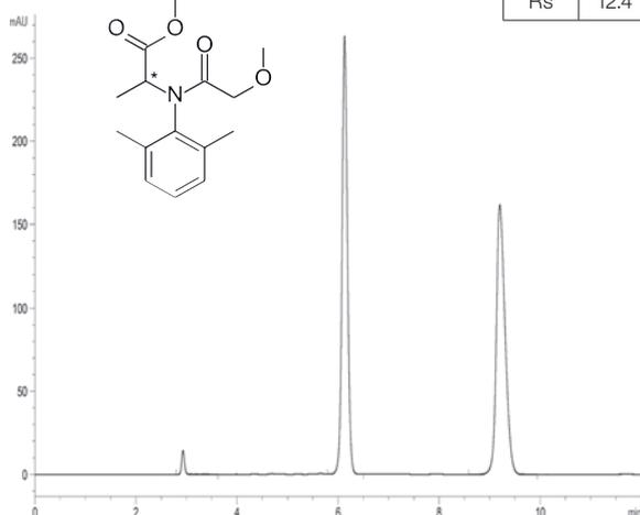
Column: CHIRAL ART Cellulose-SB (5  $\mu$ m) 250 x 4.6 mm ID
