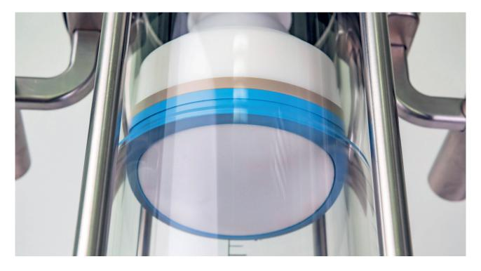
When the piston is inserted, the gasket seals permanently. This way, dead volumes are reduced to a minimum! Due to the unique construction, the gasket slides easily up and down the column.
