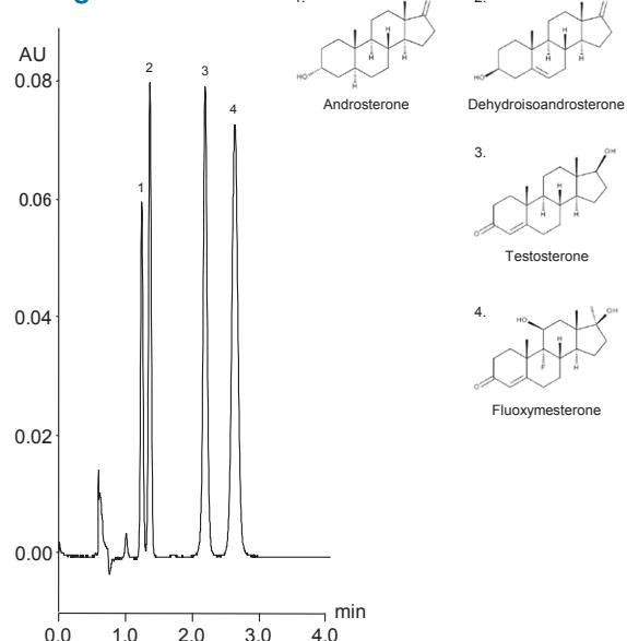
Column: YMC-Triart PFP (5  $\mu$ m, 12 nm) 150 x 4.6 mm ID
