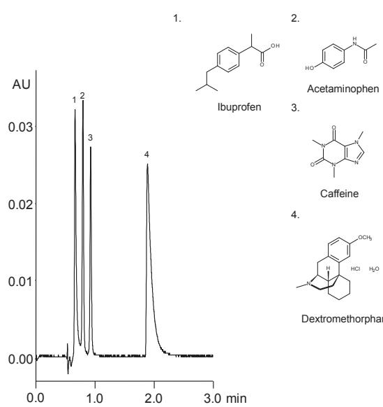
Column: YMC-Triart PFP (5  $\mu$ m, 12 nm) 150 x 4.6 mm ID
