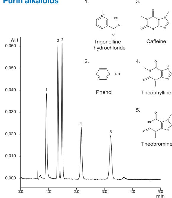
Column: YMC-Triart Diol (5 µm, 12 nm) 150 x 4.6 mm ID
