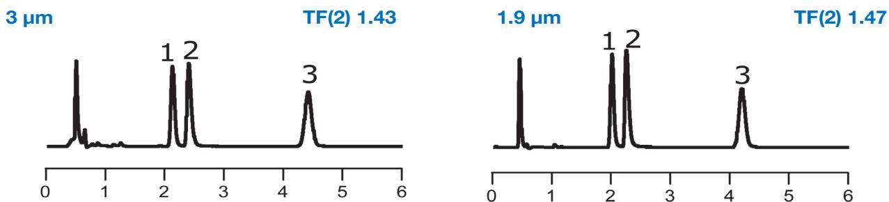
YMC has addressed this issue of method transfer. YMC-Triart columns show identical selectivity and excellent peak shapes for basic compounds for all 3.0 μm to 1.9 μm particle sizes. It allows predictable scale up from UHPLC to conventional HPLC and even to semi-preparative LC, and vice versa.
