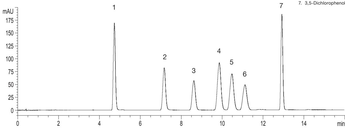
Column: YMC-Triart C18 ExRS (1.9  $\mu$ m, 8 nm) 75  $\times$  3.0 mm ID
