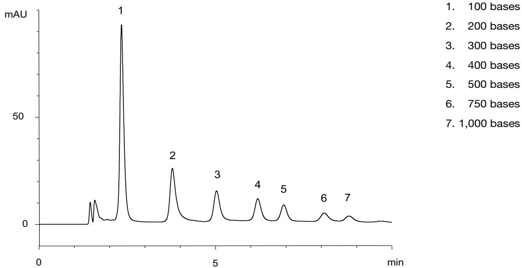
Column: YMC Accura Triart Bio C4 (1.9 µm, 30 nm) 100 x 2.1 mm ID
