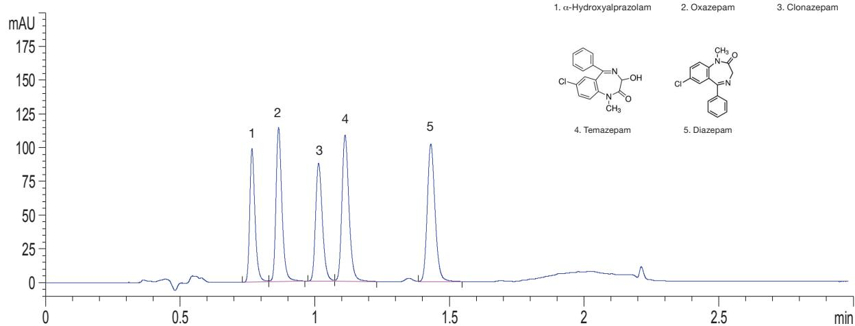
Column: YMC-Triart Phenyl (1.9  $\mu$ m, 12 nm) 100 x 2.0 mm ID
