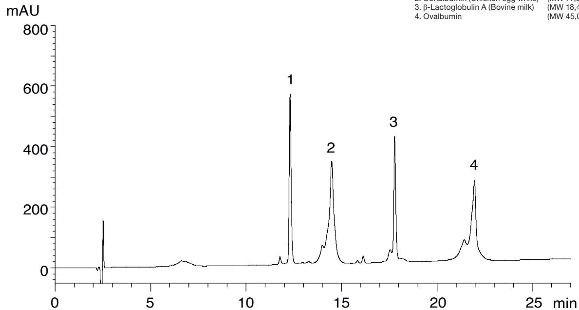
Column: YMC-Triart Bio C4 (5  $\mu$ m, 30 nm) 150 x 3.0 mm ID
