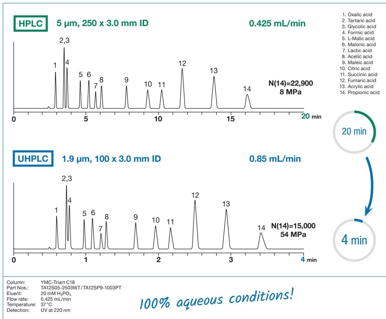
Stable under harsh conditions: pH 1–12 and temperature up to 90 °C.
