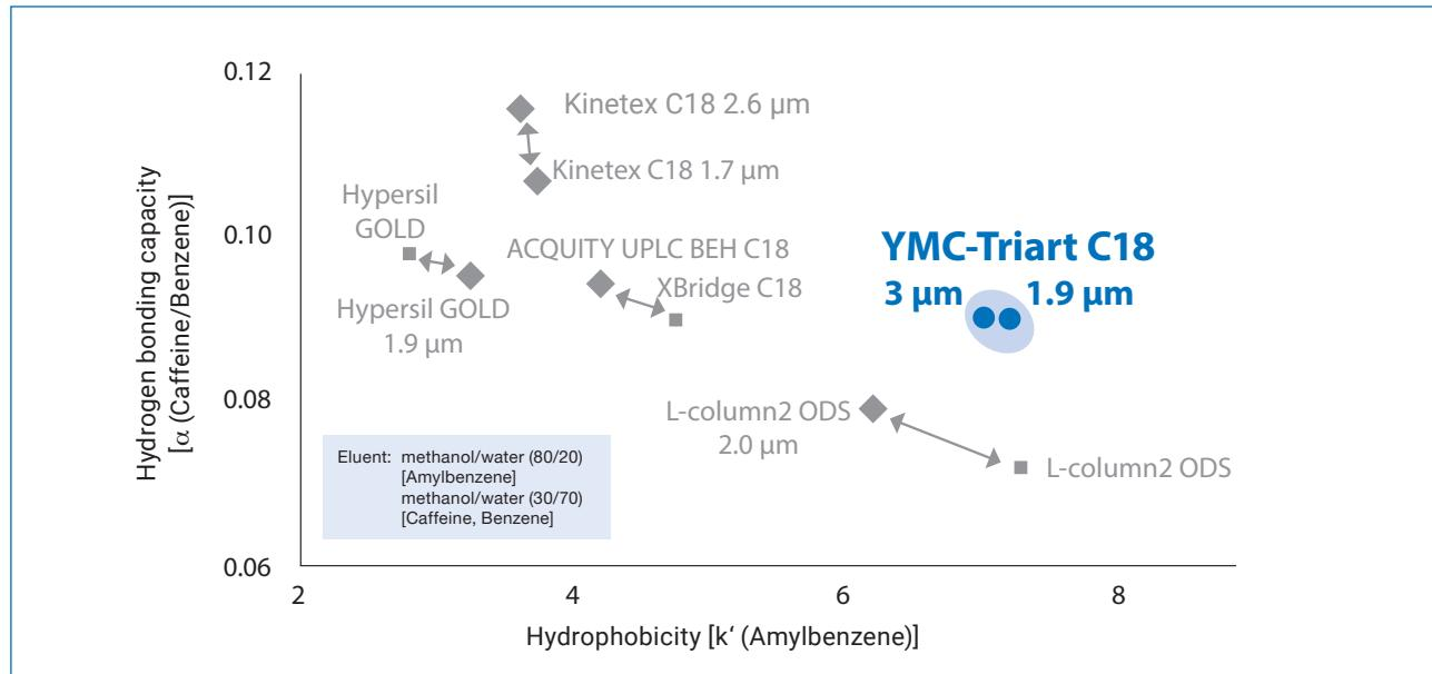
With the introduction of UHPLC, sub-2-μm particles became necessary. Therefore smaller particles have been added to existing column lines. Consequently, sub-2-μm particles may exhibit differences in chromatographic performance. By introducing YMC-Triart, YMC provides matching chromatographic behaviour for all particle sizes!
