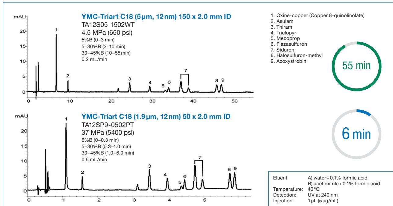
When transferring the 55 min HPLC method to UHPLC scale, the resolution remains the same although the separation time is reduced to only 6 min.
