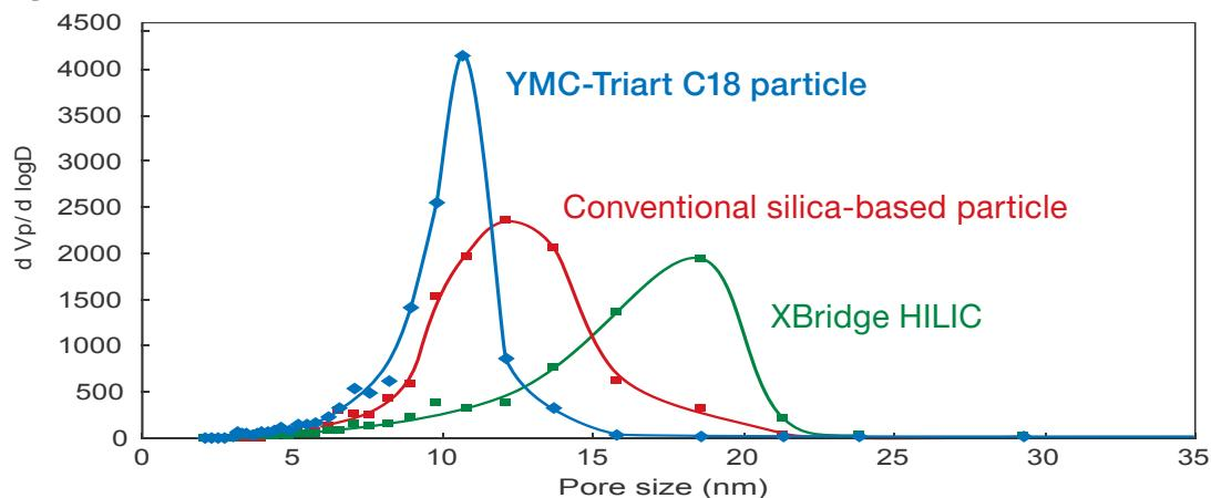
This figure shows the pore size distributions of some competitive material. Comparing the pore size distributions shows that YMC-Triart has a narrower distribution which results in sharper peak shapes.
