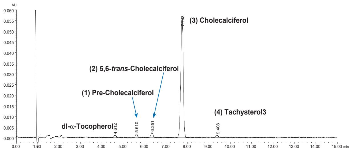
Column: YMC-Triart Diol (3 µm, 12 nm) 250 x 4.6 mm ID
