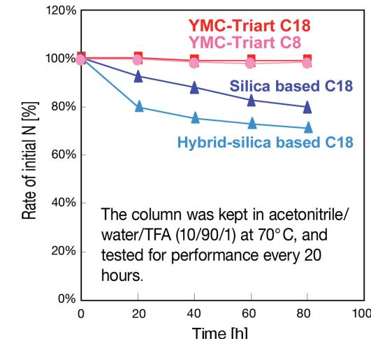
Column: YMC-Triart C18 (5 µm, 12 nm) 50 x 2.0 mm ID
