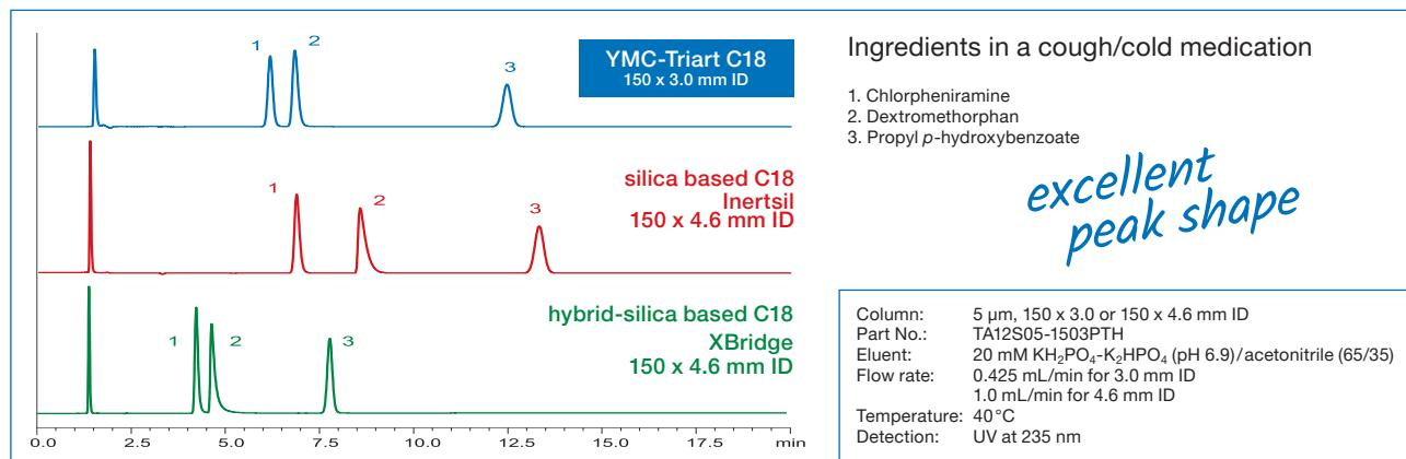
The innovative surface modification technology results in excellent peak shapes even for basic compounds that often exhibit peak tailing with conventional silica- and hybrid silica-based reversed phase columns.
