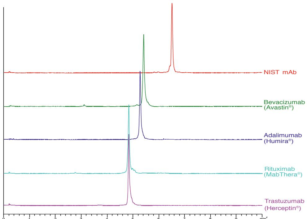
Column: YMC-Triart Bio C4 (1.9 µm, 30 nm) 50 x 2.1 mm ID
