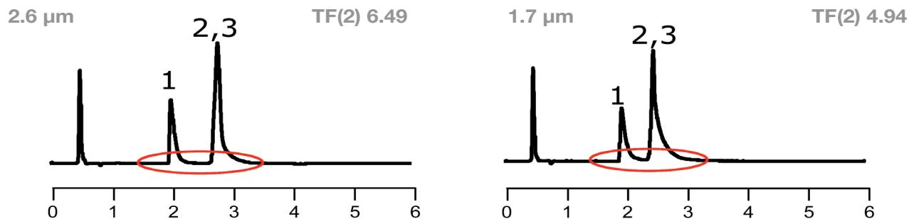
Kinetex C18 columns show significant peak tailing and have limited scalability due to lack of larger particle sizes.
