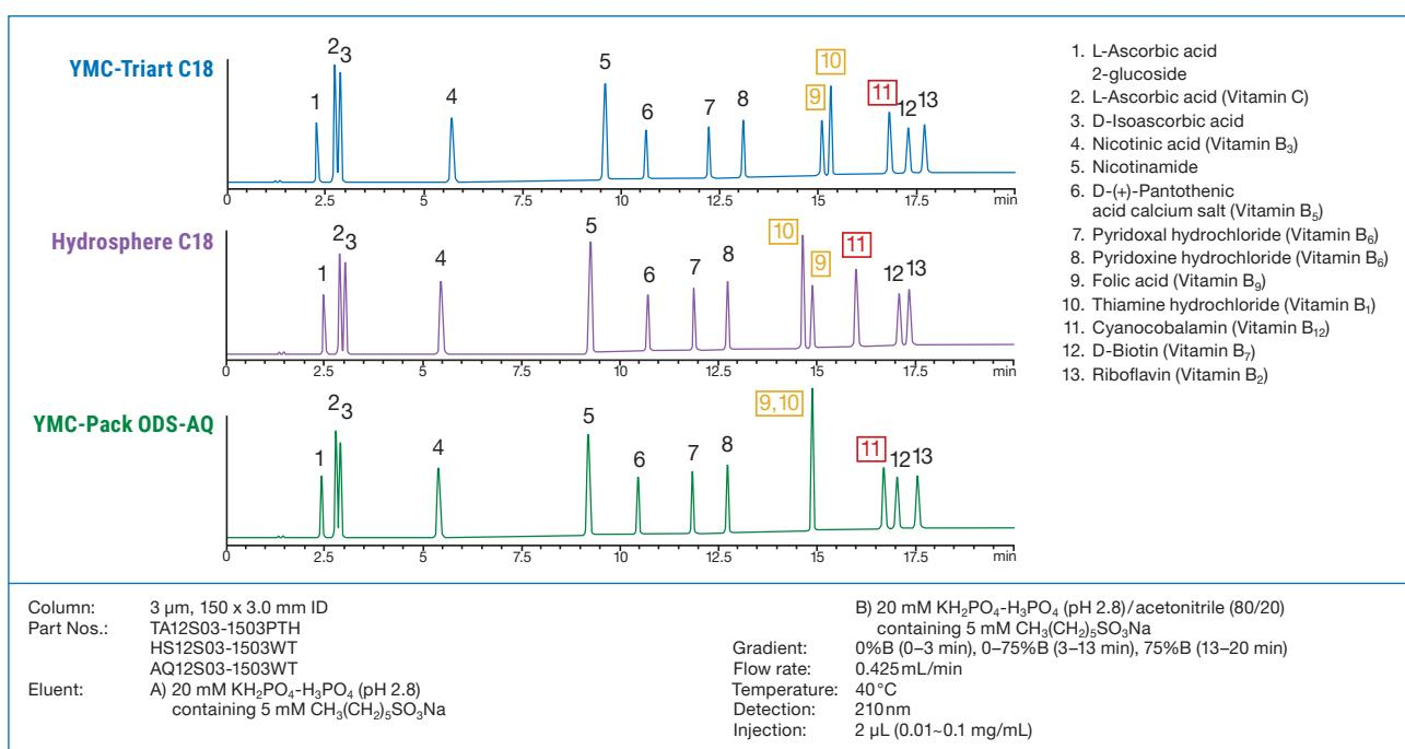
Retention behaviour of water-soluble vitamins on three YMC ODS phases which can be used with 100% aqueous mobile phases is compared. The retention times and peak elution order for folic acid (peak 9), thiamine hydrochloride (peak 10) and cyanocobalamin (peak 11) are different for the three phases due to the balance of hydrophobicity and hydrogen bonding capacity differing between the three phases.
