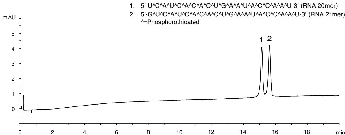
Column: YMC-Triart C8 metal-free PEEK-lined (1.9  $\mu$ m, 12 nm) 100 x 2.1 mm ID
