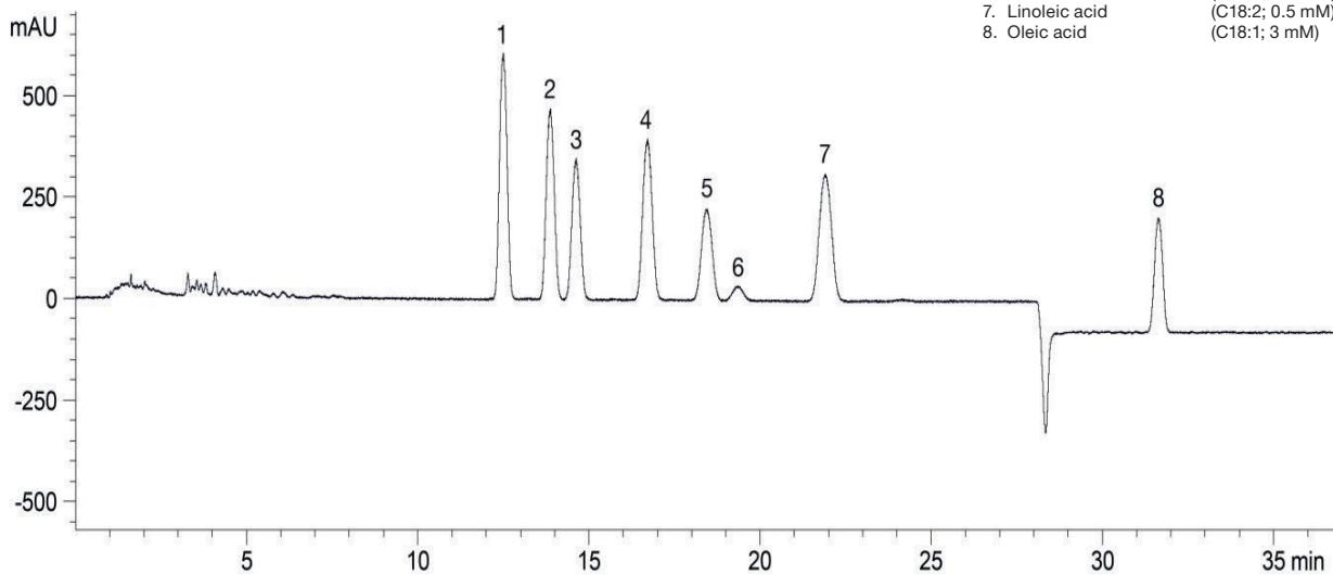
Column: YMC-Triart C18 ExRS (3  $\mu$ m, 8 nm) 150  $\times$  4.6 mm ID
