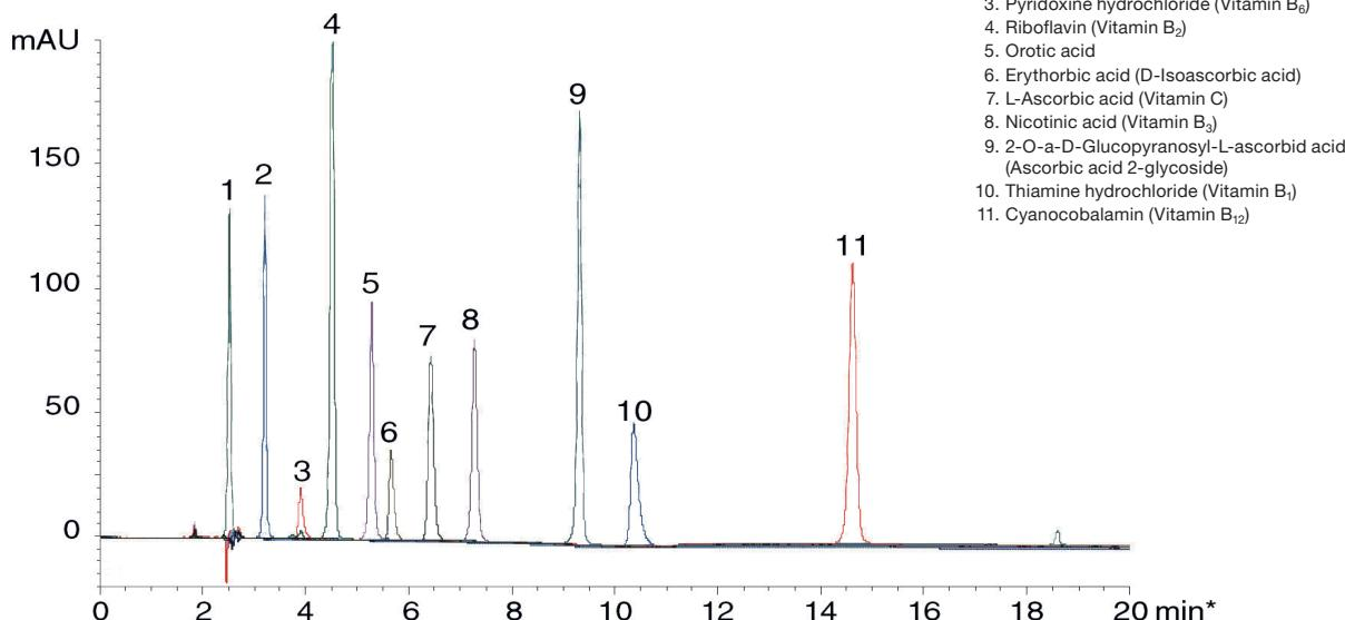
Column: YMC-Triart Diol-HILIC (5 µm, 12 nm) 150 x 3.0 mm ID
