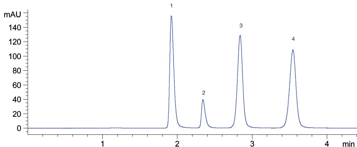
Column: YMC-Triart Phenyl (1.9  $\mu$ m, 12 mm) 100 x 2.0 mm ID
