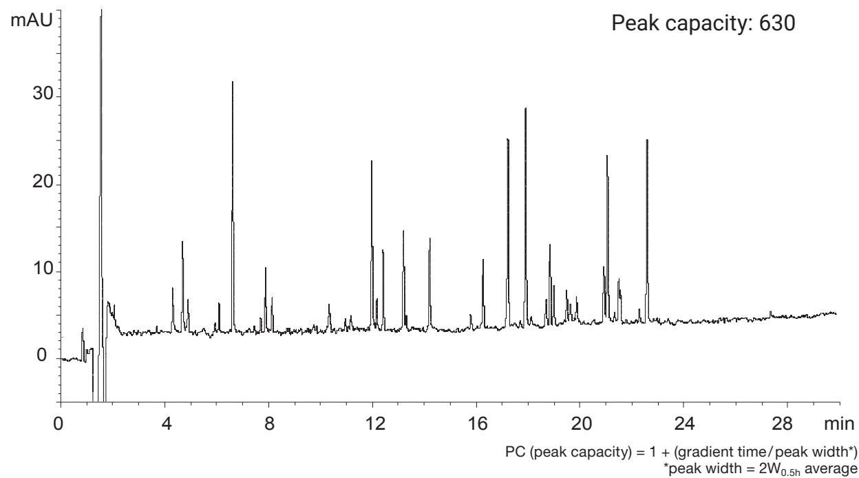
Column: YMC-Triart C18 (1.9  $\mu$ m, 12 nm) 200 x 2.0 mm ID (Two coupled 100 x 2.0 mm ID)
