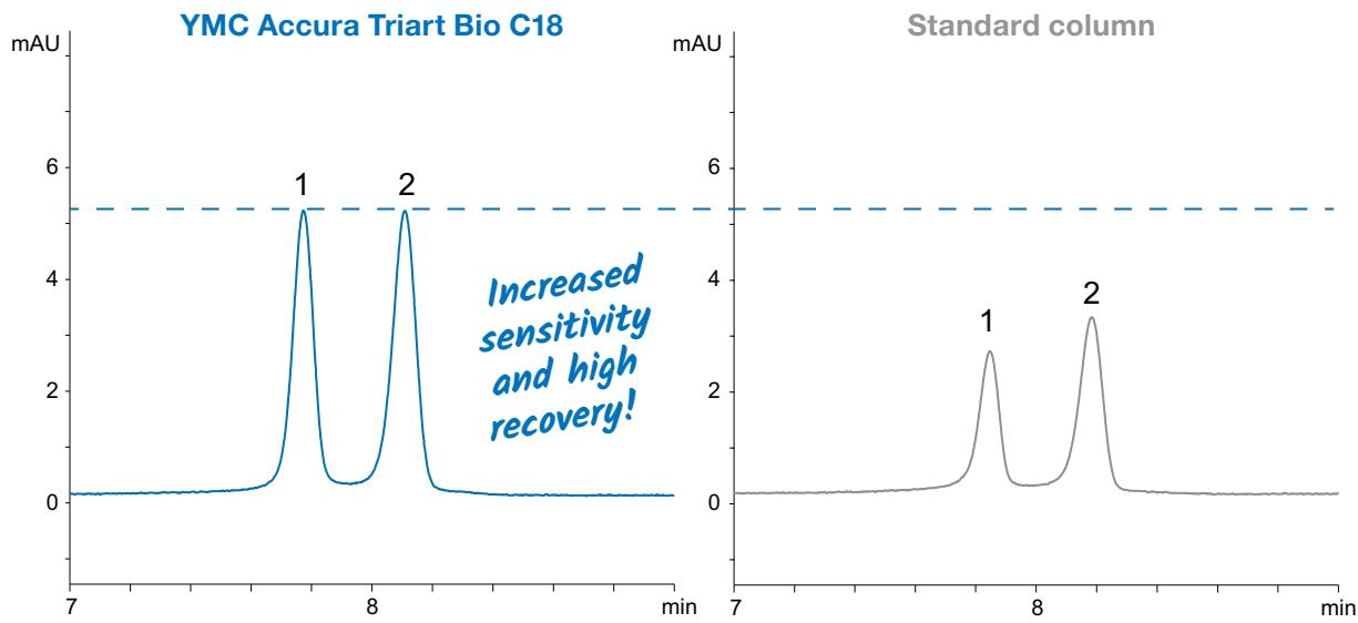
Column: YMC Accura Triart Bio C18 (1.9 µm, 30 nm) 50 x 2.1 mm ID
