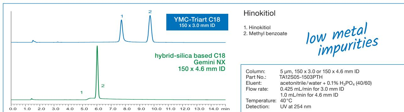
YMC-Triart phases have an extremely low level of metal impurities, much lower than conventional products, ensuring excellent peak shape for coordination compounds.
