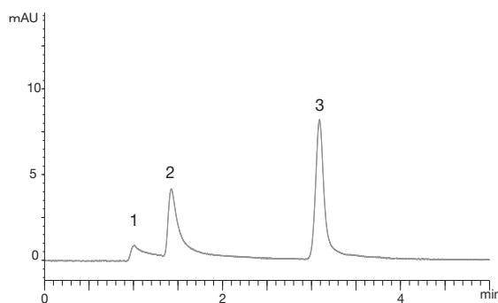
Column: YMC Accura Triart C18 (1.9 µm, 12 nm) 50 x 2.1 mm ID (bioinert hardware)
