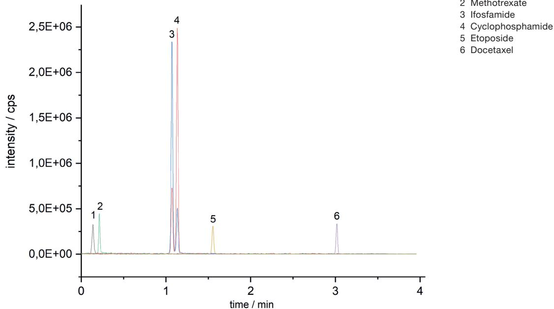
Column: YMC-Triart C18 (1.9 µm, 12nm) 50 x 1 mm ID
