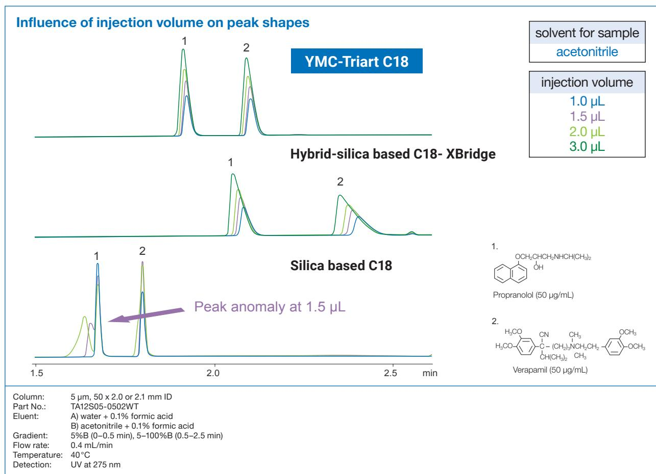
In order to prevent peak errors, there is a limit to the injection volume when a sample is injected in high elution solvents (such as 100% acetonitrile). Compared with traditional columns, more than double the injection volume can be injected into YMC-Triart columns as a result of the extremely narrow particle size distribution.
