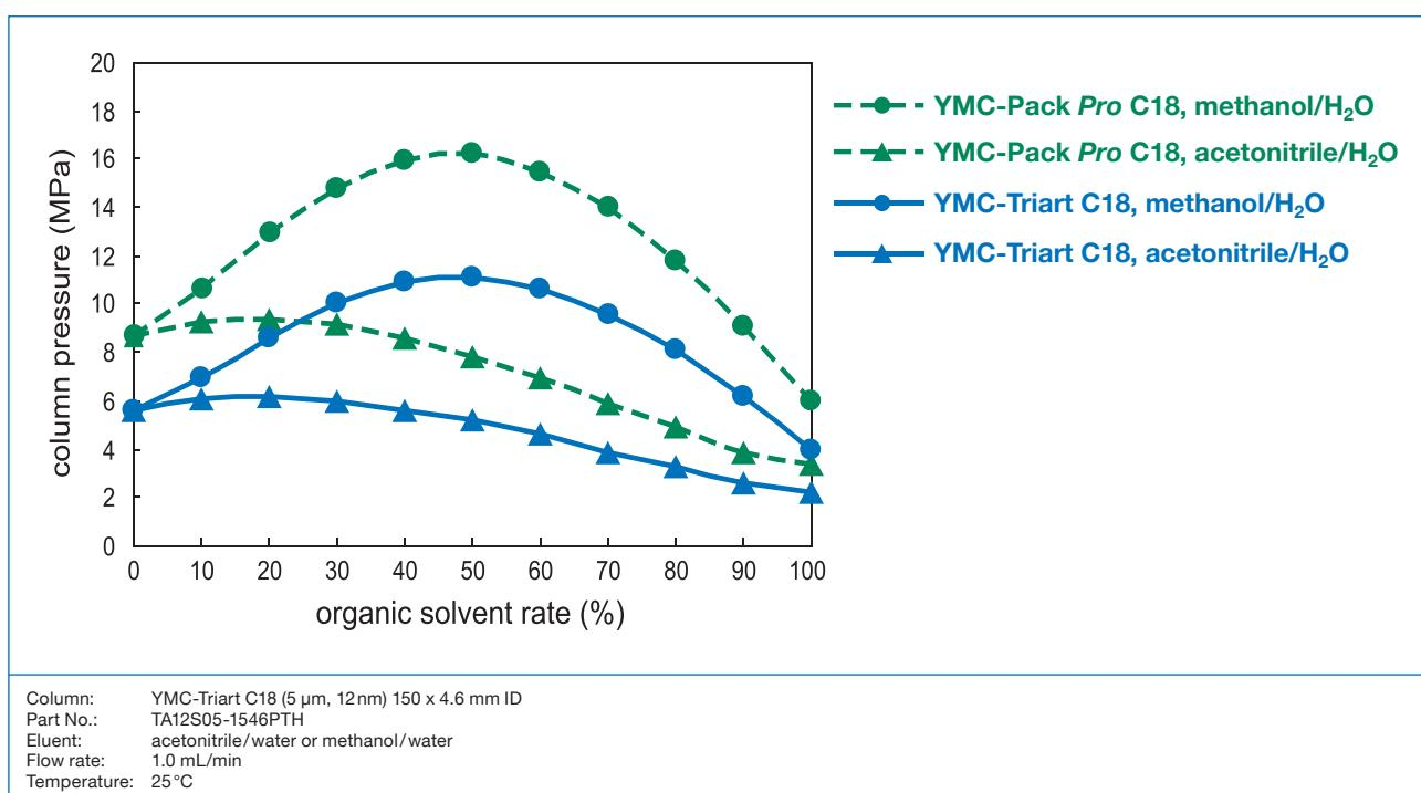
The revolutionary production technique, adapted from micro-reactor flow technology, produces a silica/organic hybrid stationary phase, with outstanding narrow pore size and particle size distributions which result in low back pressures. YMC-Triart is designed for use under a wide range of conditions. Elution with higher viscosity methanol (compared with acetonitrile), YMC-Triart generates lower pressure (approx. 30% lower than with conventional phases).
