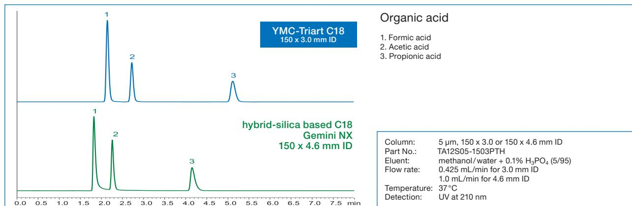
YMC-Triart phases are synthesised using methodology adapted from micro-reactor technology. This technique ensures a reduction of impurities that contribute to peak tailing during the analysis of some types of acidic compounds.
