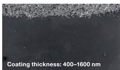
The robust bioinert coating used on **YMC Accura** hardware is 130 to 320-fold thicker making it more durable than other similar hardware concepts. A long-term inertness against sensitive substances is ensured. In order to demonstrate its robustness, a **YMC Accura** column was packed multiple times. Even though this is quite a challenge for the column surface, the coating remains unaffected (SEM\* picture: top area is bare steel for comparison). \*Scanning Electron Microscope
