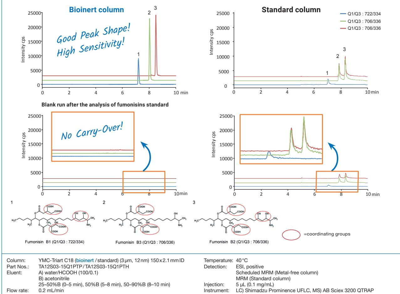
The **bioinert YMC-Triart** column showed excellent peak shapes when used to analyse fumonisins, while the regular column showed severe peak tailing due to interactions between the sample and the hardware. No carry-over was observed when using the
