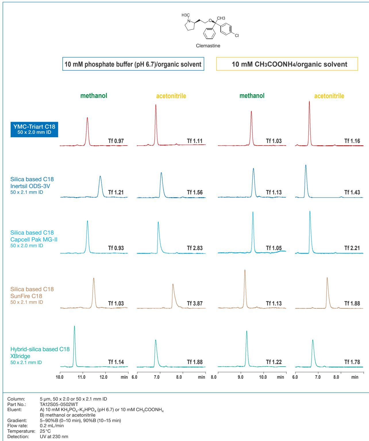
Clemastine is a well-known basic compound which readily exhibits peak tailing with conventional ODS columns. YMC-Triart C18 provides sharp separations with many different buffer/solvent compositions.
