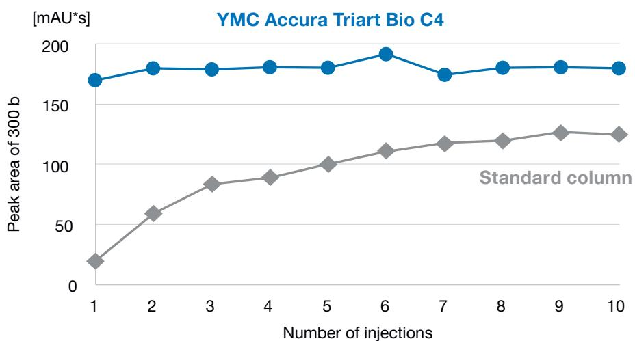
The YMC Accura Triart Bio C4 column shows stable peak areas from the first injection, while the standard stainless-steel column provides only 10% of the peak area (for the 300 base marker) with the first injection.
