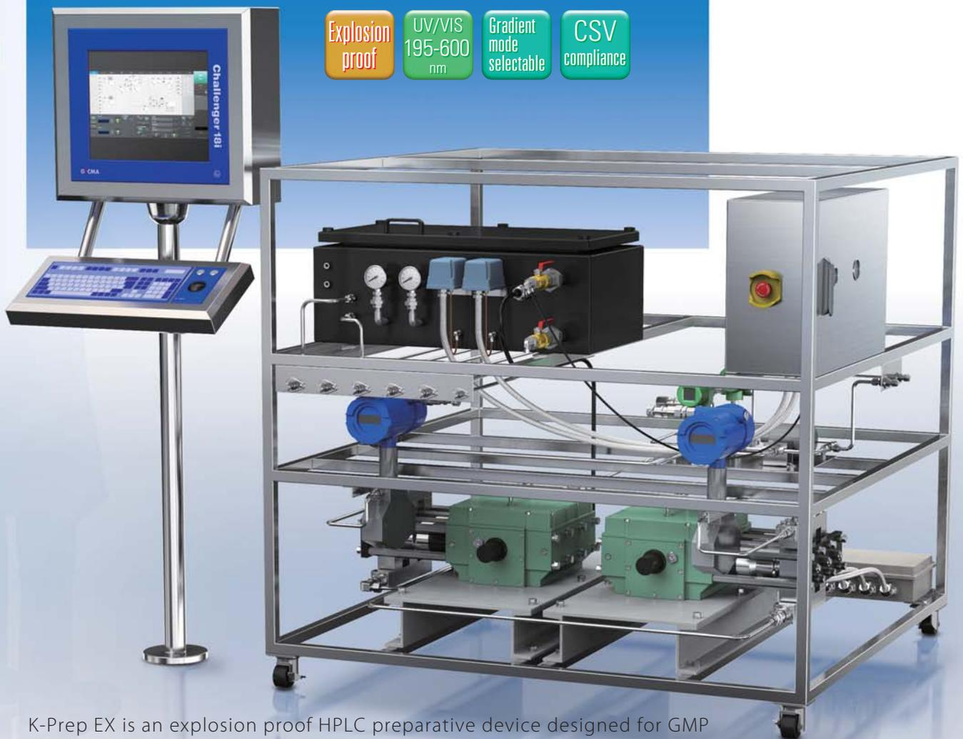
K-Prep EX is an explosion proof HPLC preparative device designed for GMP manufacturing plants.
