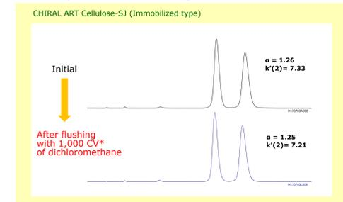
% change in selectivity ( $\alpha$ ) and capacity factor ( $k'$ ) of CHIRAL ART Cellulose-SJ after flushing with 1,000CV\* of each solvent at 40°C
