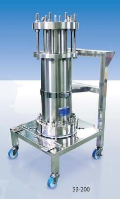
SB products are statically compressed cost effective preparative columns which enable convenient self-packing. Tightening screw bolts of the upper flange yields a compressed packing bed. Not only dry packing but also wet (slurry) packing is possible by attaching a column packing extender (optional).
