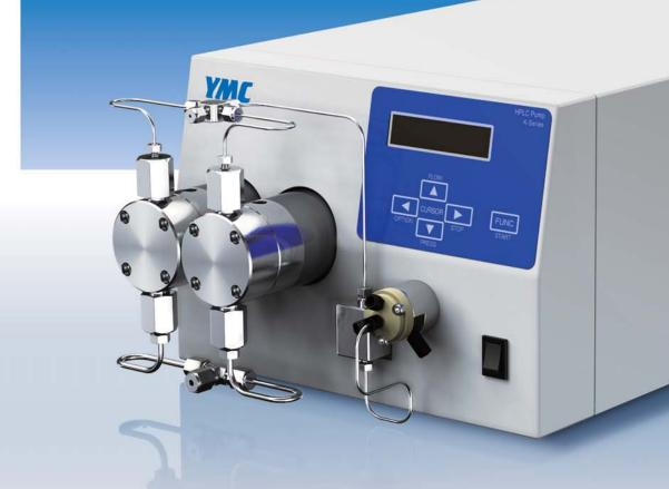
K series pumps are designed for preparative chromatography employed worldwide for simple and demanding applications. K-Prep dual reciprocating plungers and the high precision servo motor enable highly-accurate pumping with less pulsation.
