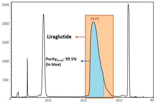
Figure 1: The purification of liraglutide with YMC-Triart Prep C18-S (10 μm, 12 nm, 250 x 10 mm ID).
