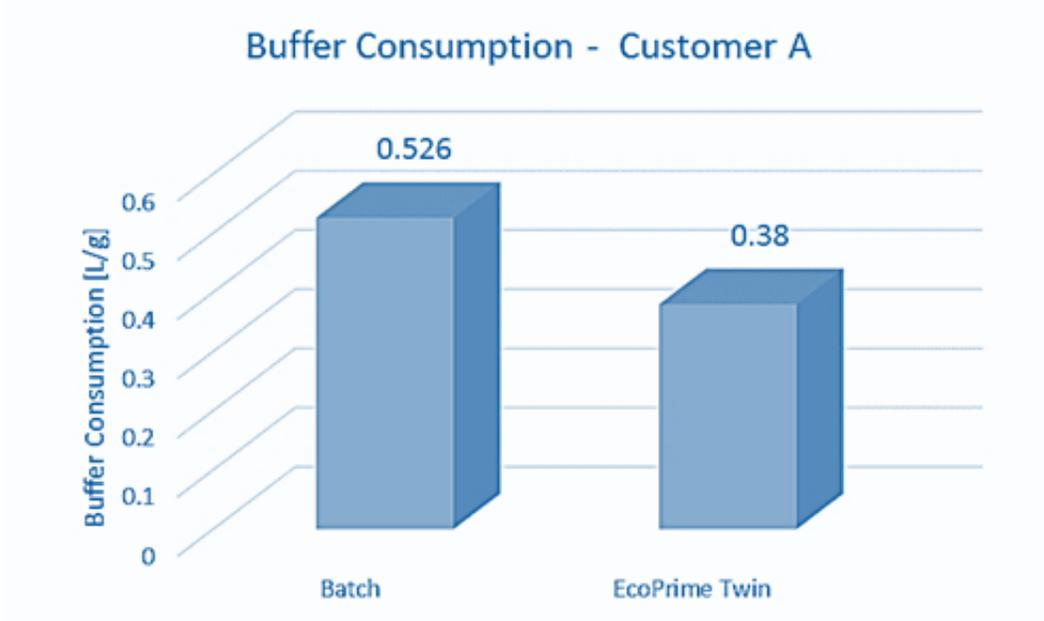
Triple productivity or 67% less resin and ~30% reduction in buffer consumption
