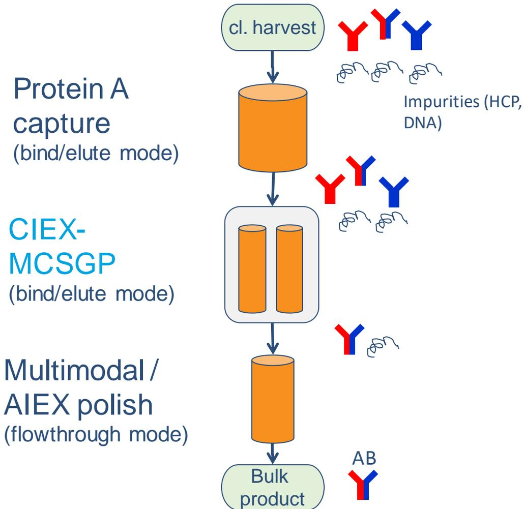
Purify bispecific antibody AB from PER.C6 harvest, remove aggregates, HCP, DNA, and parental antibodies AA and BB
