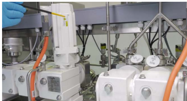
Figure 8. The system achieves extraordinary precision and accuracy due to unique fluid engineering design and exclusive LEWA intellidrive technology. The servo motor controls the buffer flow with digital precision and allows the system to achieve dilution factors of 1:150.
