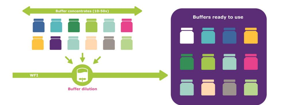
Alternatives to traditional buffer preparation include ready to use buffers, buffer stock blending, and buffer dilution. Buffer dilution can answer these pain points through the combination of buffer concentrates (up to 50X), a buffer dilution skid that prepares ready to use solutions with accuracy and precision, and single use components for distribution throughout the plant. This combination can increase plant flexibility, while reducing classified floor space, labor and CAPEX requirements.
