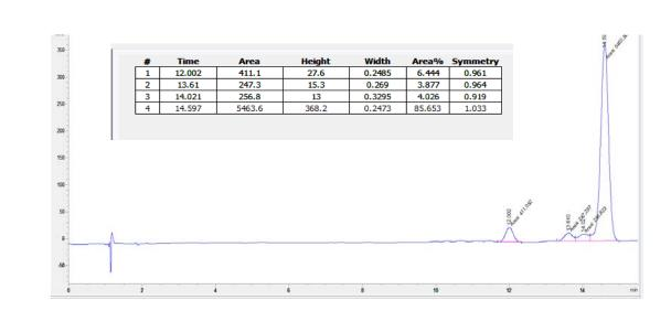
With data from the Batch Fraction Analysis Table, expected purity and yield estimates can be made for different batch methodology pools. Purity estimates can also be made for MCSGP methodology based on this batch method data.
