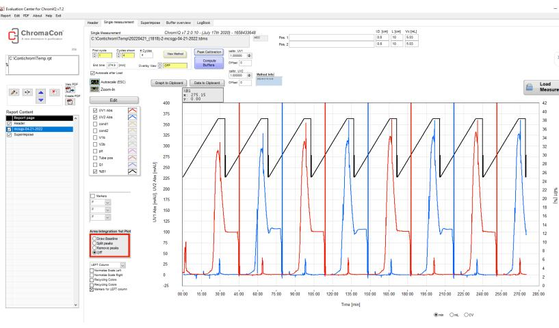
The MCSGP data can also be displayed as an overlay of the different cycles. The shaded areas represent the portions that are the early eluting recycled portion, the collected portion and the late eluting recycled portion.
