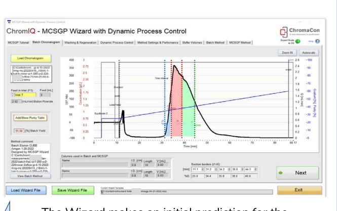
The Wizard makes an initial prediction for the chromatographic method. Adjustments can be made to sample loading, flow rates, column washes and equilibration steps parameters.
