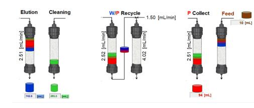
The left column running a sample while the right column is being cleaned. Recycling the impure early eluting portion. Collecting the pure portion and adding more feed to the second column. Recycling the impure late eluting portion. The next step would be the right column running a sample while the left column is being cleaned.
