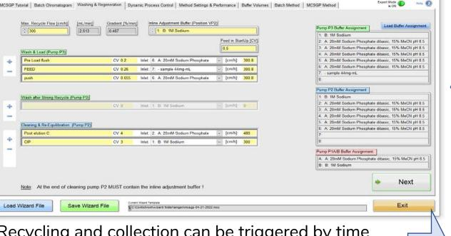
Recycling and collection can be triggered by time or by detector response. The recycled solutions are diluted before entering the next column. The amount of dilution is set within the Wizard.
