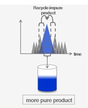
An MCSGP process collects the pure portion of the desired peak. The portions with early and late impurities are sent to a second column while adding more feed material and the purification continues
