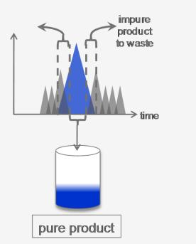
A typical batch process collects the pure portion of the desired peak. The portions with early and late impurities are discarded or retained for later reprocessing
