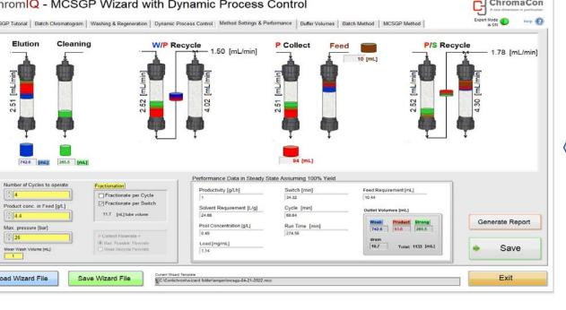
The Wizard calculates the total amount of sample feed, buffers and eluents used for the MCSGP method and for the associated startup and shutdown methods.
