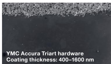
The robust bioinert coating used on YMC Accura hardware is 130 to 320-fold thicker making it more durable than other similar hardware concepts. A long-term inertness against sensitive substances is ensured. In order to demonstrate its robustness, a YMC Accura column was packed multiple times. Even though this is quite a challenge for the column surface, the coating remains unaffected (SEM\* picture: top area is bare steel for comparison).
